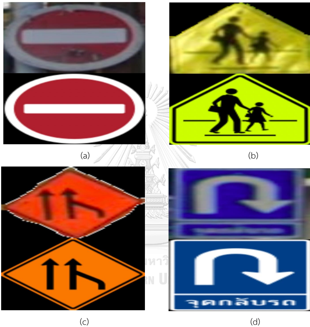
Figure 4.3 Example of template matching results of Thai traffic signs (a) Regulatory class (b) Warning class (c) Construction class (d) Guide class
