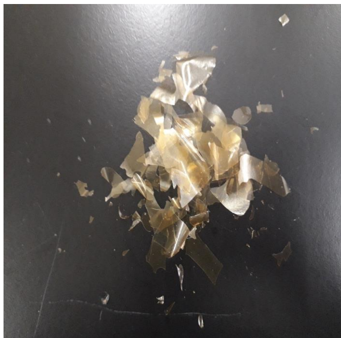
Figure A1 The brittle characteristic of EFB CMC films due to low glycerol concentration (less than 0.50% v/v).
