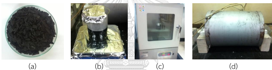
Figure 3.9 Ni/char catalyst was prepared by the impregnation method (a) char support (b) impregnation with \text{Ni}(\text{NO}_3)_2 \cdot 6\text{H}_2\text{O} (c) drying (d) calcination.
