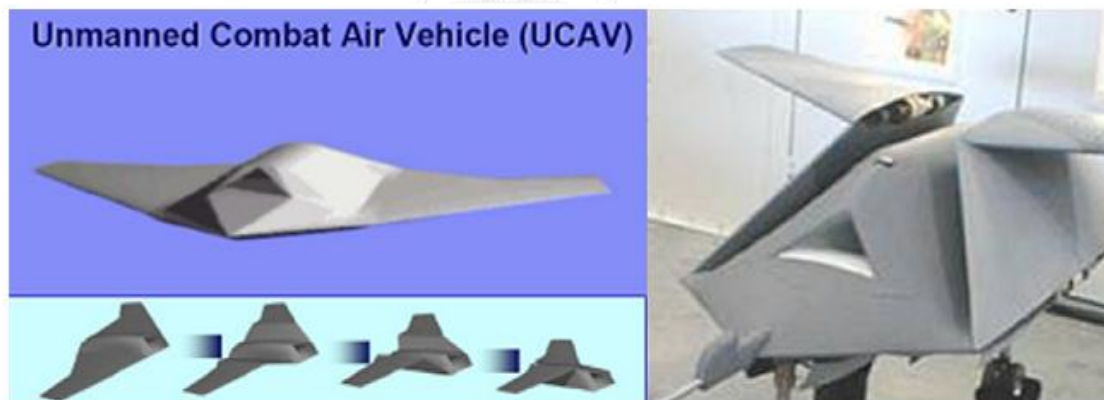
Figure 2.7 Shaped morphing wings produced by Lockheed Martin [3, 37].
