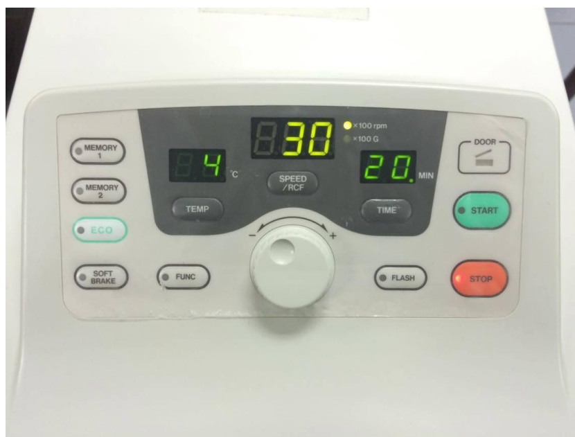
Figure A.4 Centrifugation at 4 degree Celsius and 3000 rpm for 20 minutes
