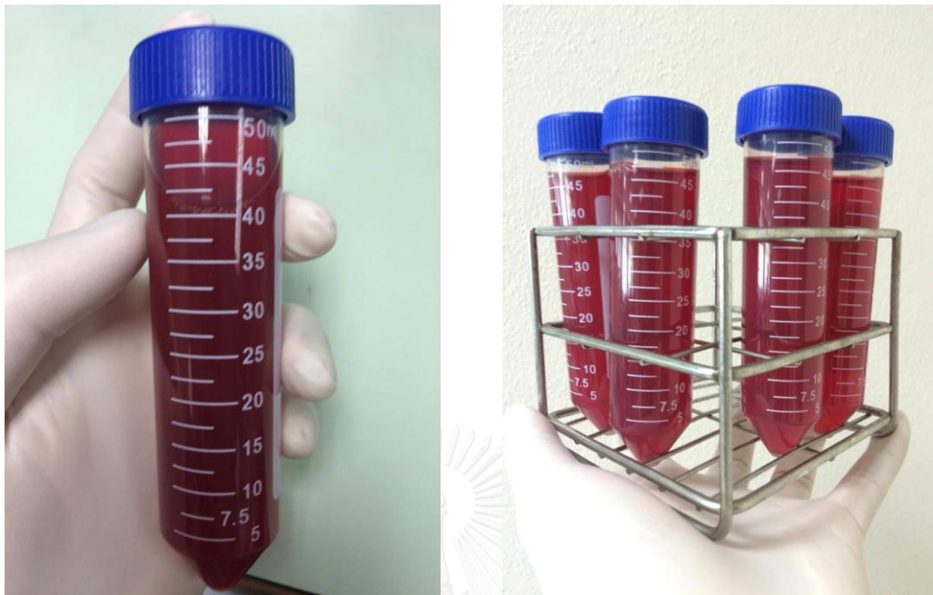
Figure A.2 Putting 3 ml of Canine blood with RBC lysing solution together into a 50 ml plastic centrifuge tube
