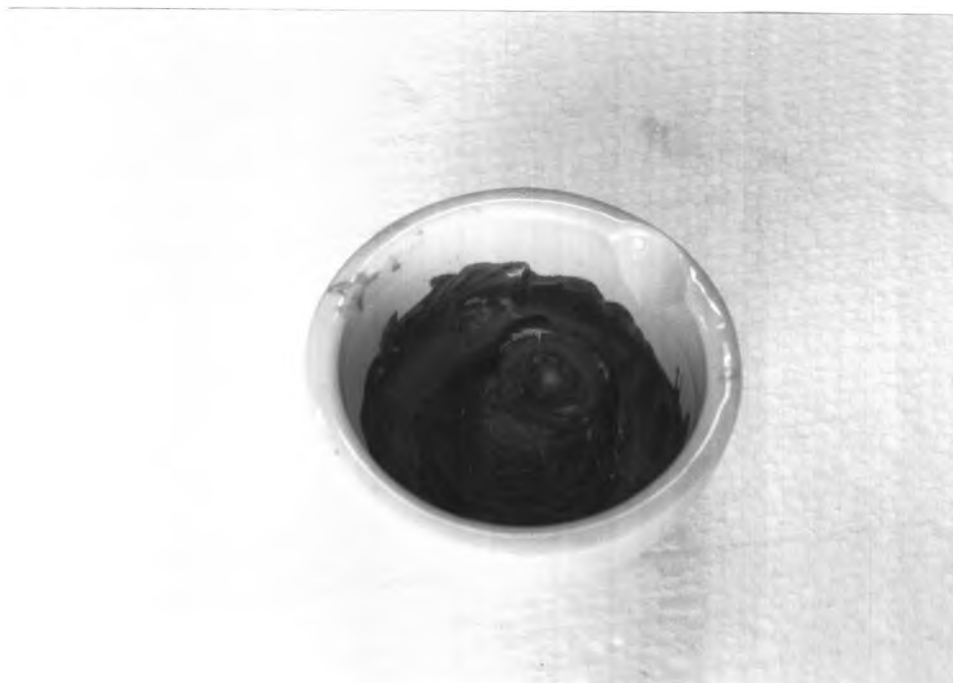
c. Mixed-Grind of the precipitate and \text{CrO}_3 from the oven
