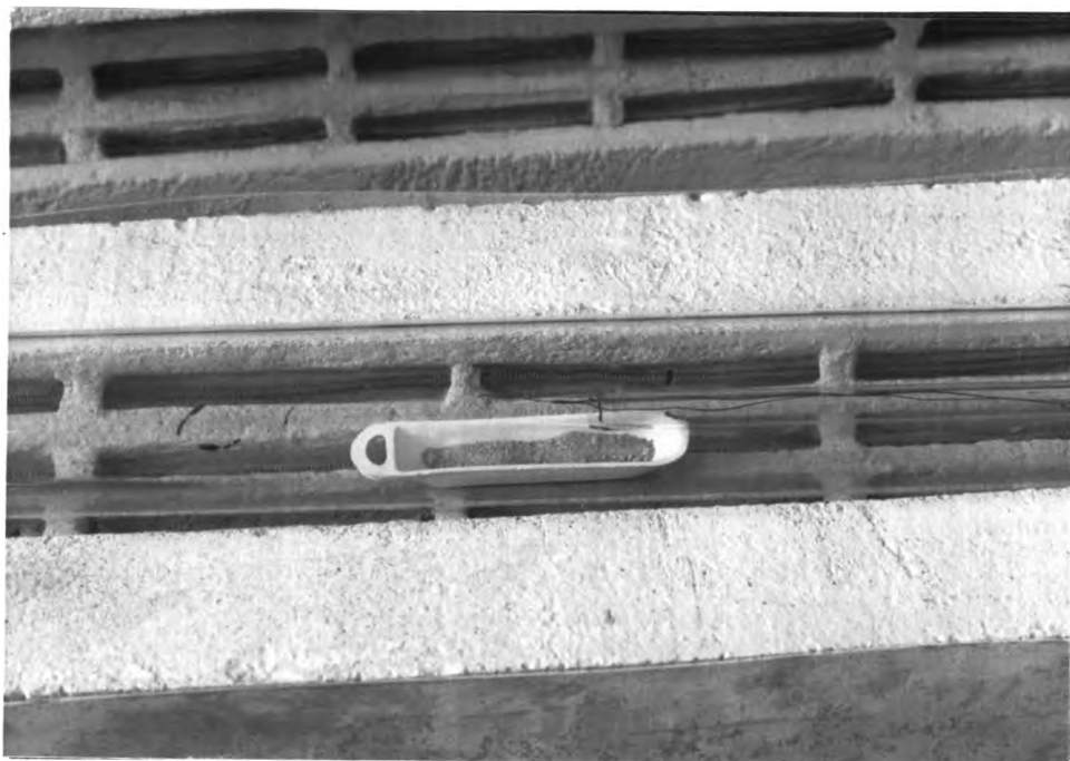
Figure 4.7 Prepared Catalyst on the boat in the Reduction Furnace
