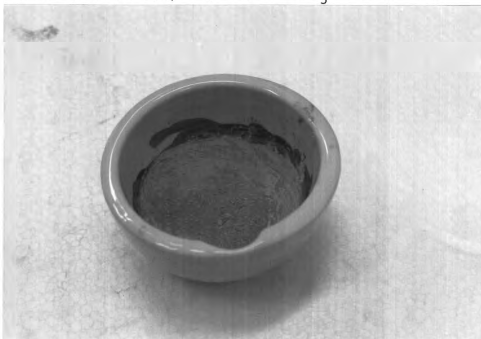
d. Mixed-Grind of about 5 gm. \text{CuO}/\text{ZnO}/\text{Cr}_2\text{O}_3 with the atomic ratios of \text{Cu}:\text{Zn}:\text{Cr} = 31:38:10
