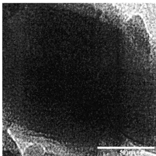
Figure 4.6 Crystal lattice of nanosized ZSM-5 formed at 150 °C for 6 h after 5 h aging time, using CXDI as hard template.
