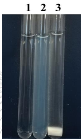
Figure 46 Comparison of solubility of three glucan polymers in water. Tube 1; 1% (w/v) of dextran polymer of Leuconostoc spp. (Sigma), tube 2; 1% (w/v) of WTALT polymer, and tube 3; 1% (w/v) of insoluble mutan polymer of S. sorbinus . The polymers were suspended in water and stood still for 15 min.
