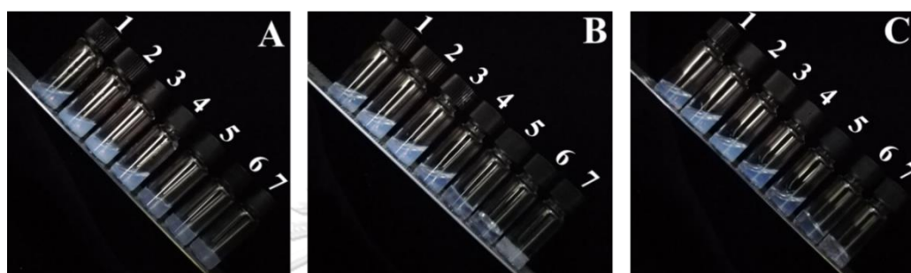
Figure 48 Comparison of solubility of WTALT (A), \Delta 3SHALT (B) and \Delta 7SHALT (C) polymers. Tubes no. 1-7 represent polymer in concentrations of 1, 2.5, 5, 10, 15, 20 and 25 % (w/v), respectively.
