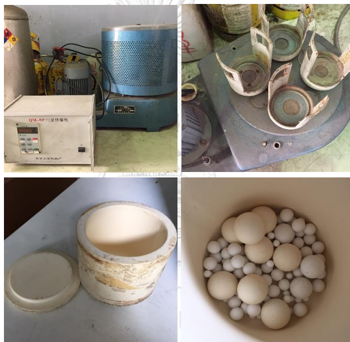
Figure 3.1 Planetary ball mill with ceramic chamber and balls (QM-BP, NANJING, Jiangsu, China)
