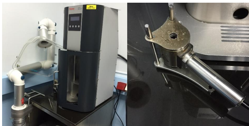
Figure 3.3 Minijet injection machine (HAAKE MiniJet II, Thermo, Scientific, Karlsruhe, Germany)
