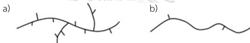
Figure 2.2 The structure of a) LDPE with long and short chain branching and b) HDPE with short chain branching only
