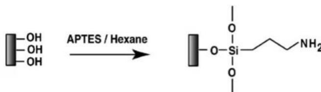
Figure 3.1. Reaction of functionalizing APTES on HAp nanoparticles.
