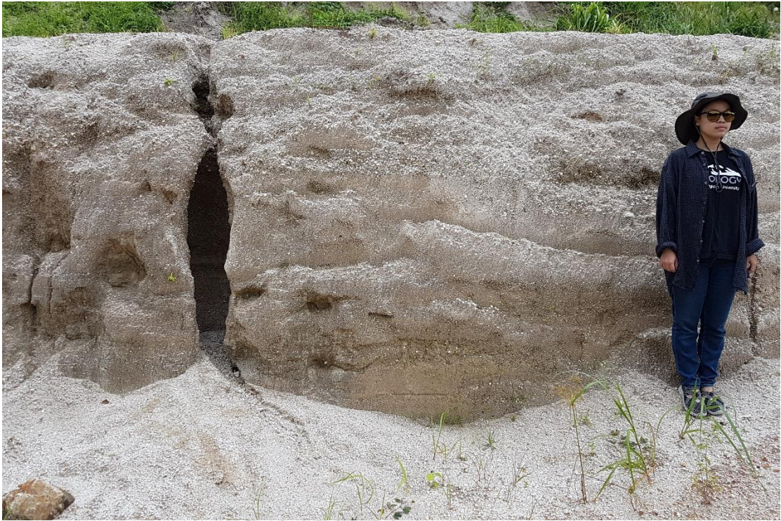
Figure 11 Heavily altered and weathered granitic rock at Takua Pit Thong mine. Note that this is NOT a pile of soil because this can be seen all over the mining area
