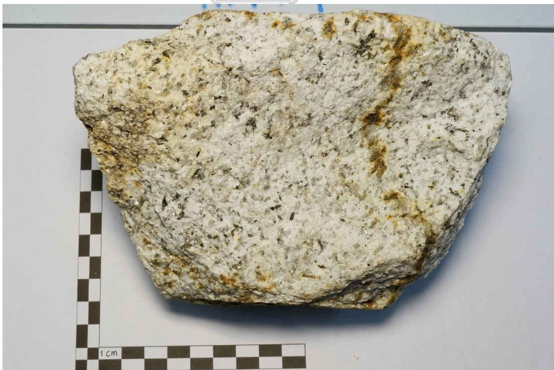
Figure 43 Sample TK4-1-4, representing tourmaline-biotite granite, one of equigranular granite
