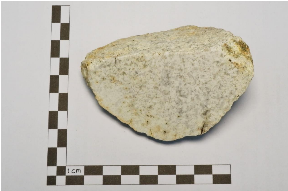
Figure 42 Sample TK1-1-5 from Takua Pit Thong area, representing equigranular granite
