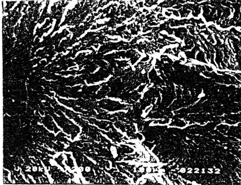
Figure 3.12 SEM photograph of impact fracture surface showed mirror region and hackle lines of Nylon 6,6.
