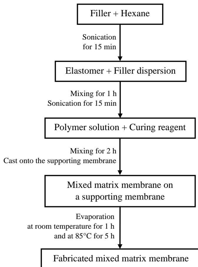
**Figure 3.2** Flow diagram of the MMM preparation.
