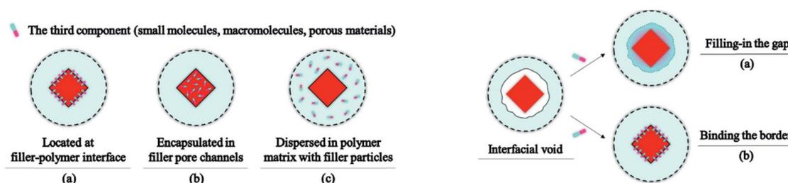
**Figure 2.5** Schematic illustration of possible existing forms of the third component in solid-liquid-polymer MMMs and interfacial void healing by the third component (Guo *et al.*, 2019).
