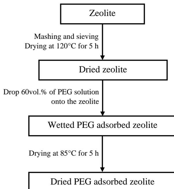
**Figure 3.1** Flow diagram of the PEG adsorbed zeolite preparation.
