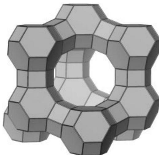
**Figure 2.2** Framework structure for FAU zeolite formed by linking sodalite cages through double six-rings (Broach, 2010).
