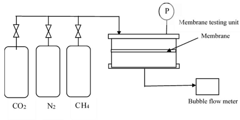
**Figure 3.3** Schematic diagram of the single gas permeance measurement.
