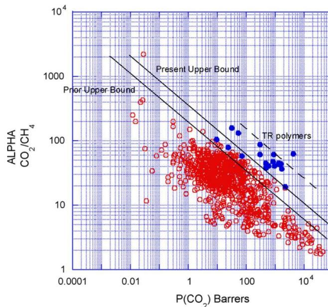
**Figure 2.1** The Robeson's upper bound of CO<sub>2</sub> and CH<sub>4</sub> (Robeson, 2008).
