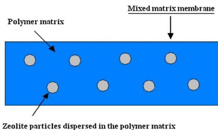
**Figure 2.3** Schematic of the mixed matrix membrane (Bastani *et al.*, 2013).
