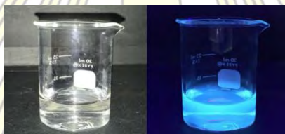
Figure 3.1 Photographs of the QGDs solution which were taken by smartphone under visible light (left) and under black light (right).
