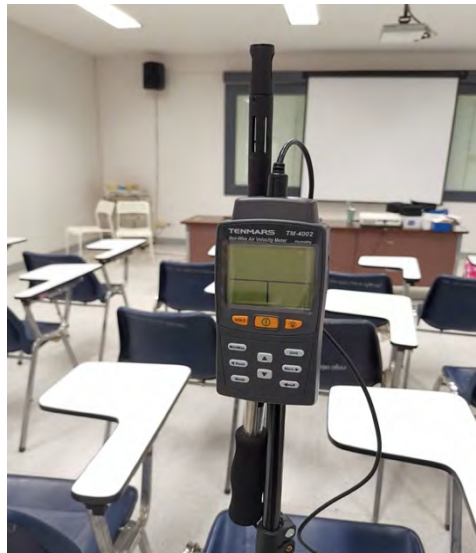
Figure 3.3 The Tenmars Model TM-4001 for the measurements of air velocity inside the classroom
