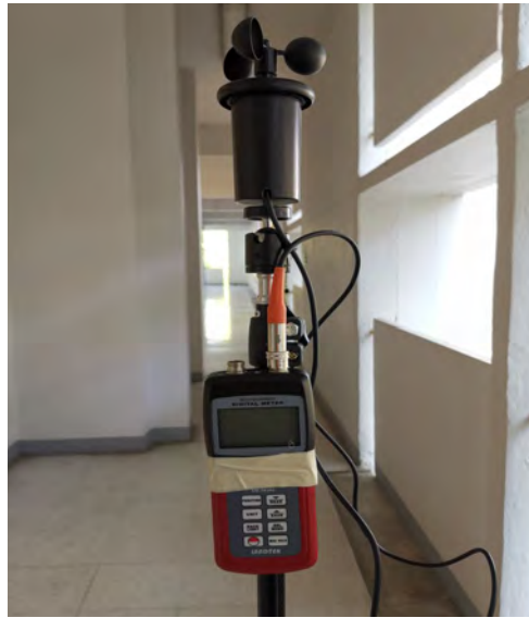
Figure 3.4 The Digital Anemometer Model AM-4836C for the measurements of air velocity outside the classroom
