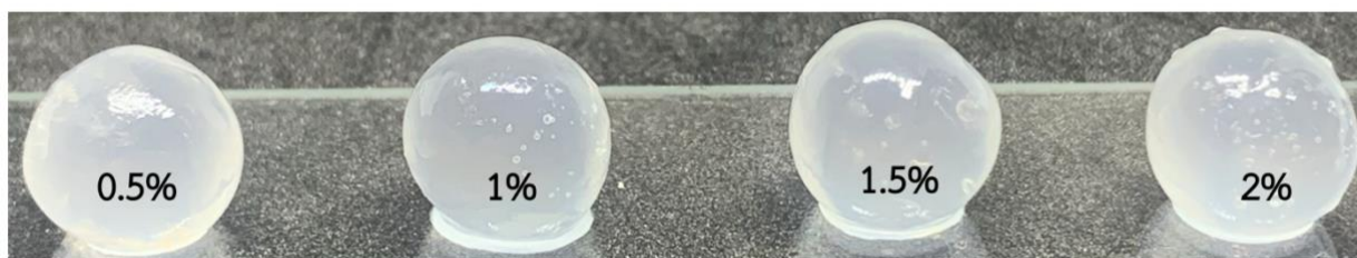
Figure 3.9 Polymeric beads formed by using various concentration of sodium alginate.
