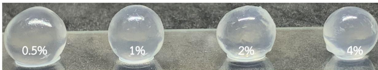
Figure 3.12 The morphology of the polymeric bead which prepared by various concentration of calcium lactate from 0.5 to 4 %(w/v).
