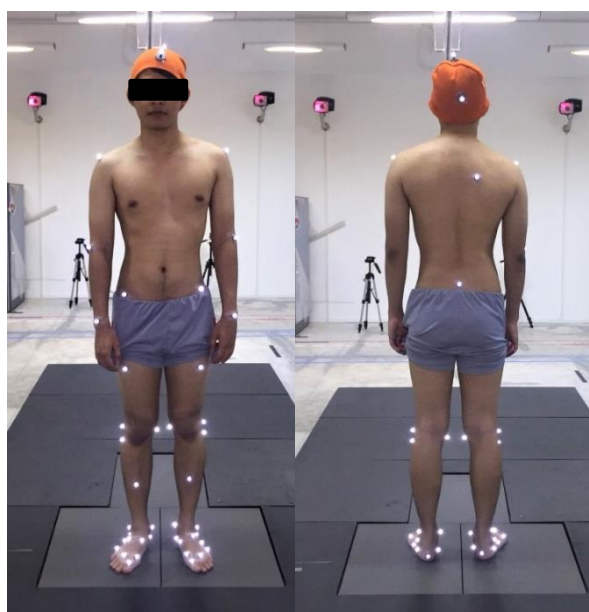
Figure 6.2 Marker placement based on the Helen-Hayes model and the multi-segment foot model
