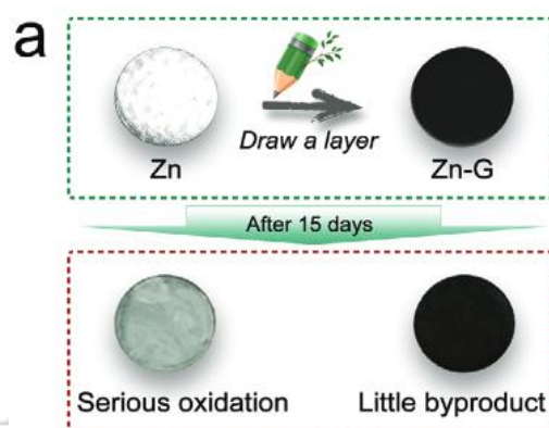
Figure 2.7 Schematic illustration of the modification process and the stability in 2 M \text{ZnSO}_4 electrolyte of Zn and Zn-G anodes. [7]
