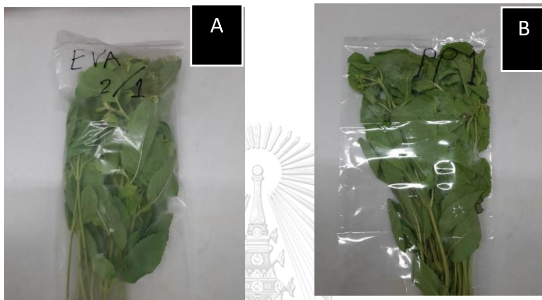
Figure 4.8 Example of basil 80 g packed in test packaging A (EVADSM) and B (commercial perforated PP).
