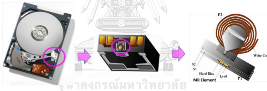
Fig. 1.1. Hard drive components and write/read heads (1).
