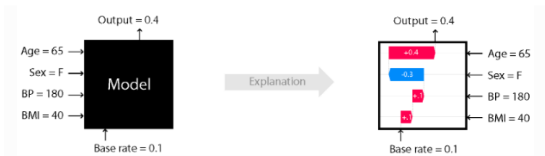
Figure 5: A toy example showing the feature impacts (SHAP values) on the model output.
