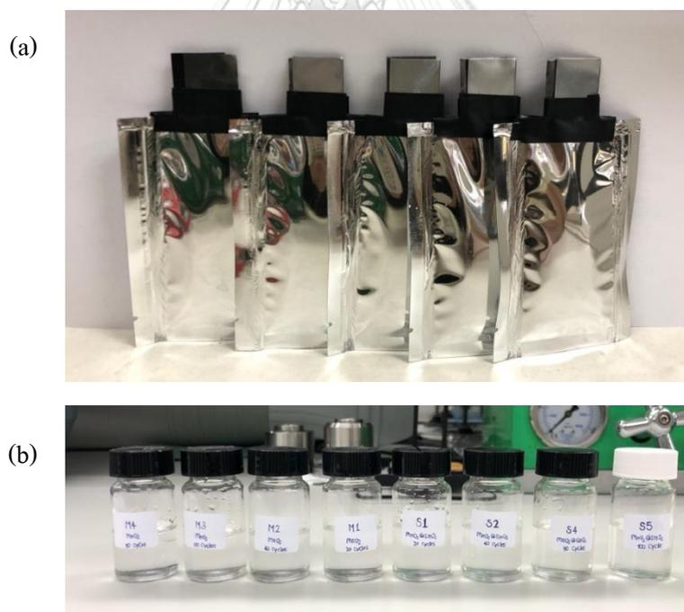
**Figure 4.11** (a) Pouch cell of the Zinc- $\text{MnO}_2$  and Zinc- $\text{MnO}_2@/\text{SnO}_2$  (0.3MS) batteries with positive electrode processed, (b) Electrolytes solution from pouch cell after charge/discharge 20, 40, 60, 80 and 100 cycles,
