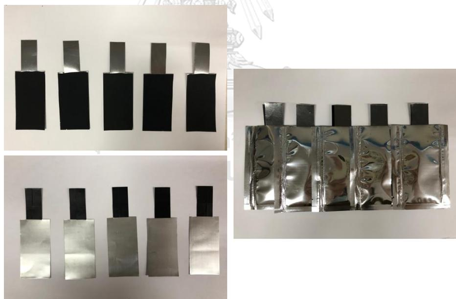
*Figure 3.2 The components of a pouch cell battery.*
