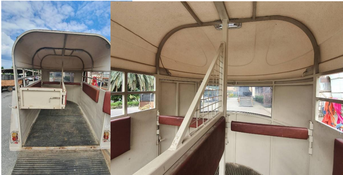
Figure 2: The ramp and the interior design of the Horse Trailer, which also shows the horse partition divider inside the Horse Trailer.
