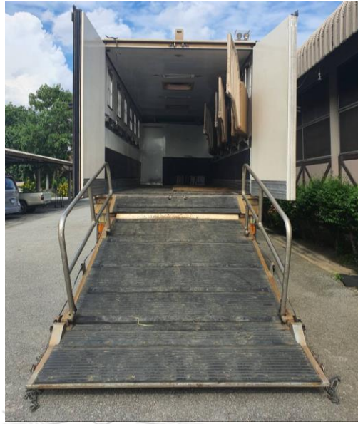
Figure 6: The ramp and the interior Horse Air-Conditioning truck.
