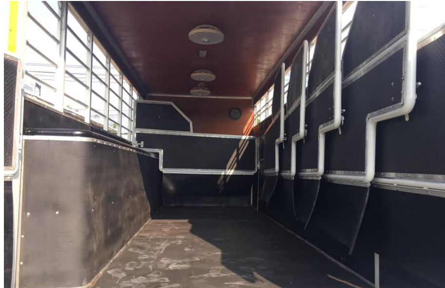
Figure 4: The interior design of the Horse Non-Air-Conditioning truck that shows the horse partition divider inside the truck.
