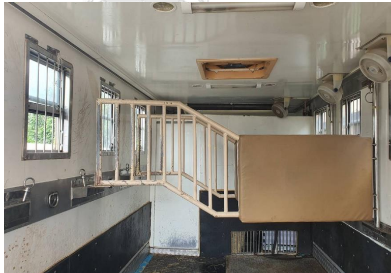
Figure 7: The interior of the Horse Air-Conditioning truck, which show horse partition divider and air-conditioning inside.
