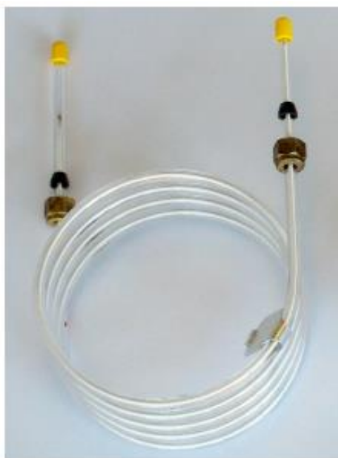
Figure 2.13 Packed column of gas chromatography (Piantanida and Barron, 2014).
