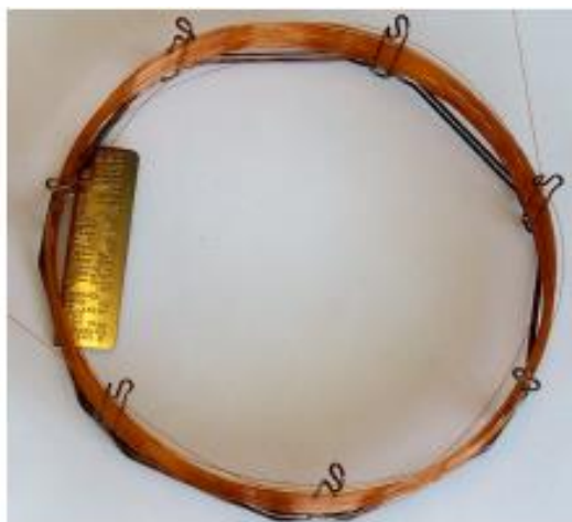
Figure 2.12 Capillary column of gas chromatography (Piantanida and Barron, 2014).
