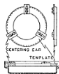
FIG. X2.3 Template Suitable for Use in Making the Wax Seals on Test Dishes
