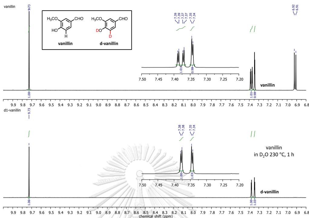
**Figure 3.5** <sup>1</sup>H NMR spectra of vanillin before and after hydrothermal HDx
