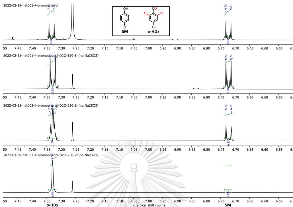
**Figure 3.26**  $^1\text{H}$  NMR spectra of deuteration of 4-bromophenol in the absence of  $\text{Na}_2\text{SO}_3$
