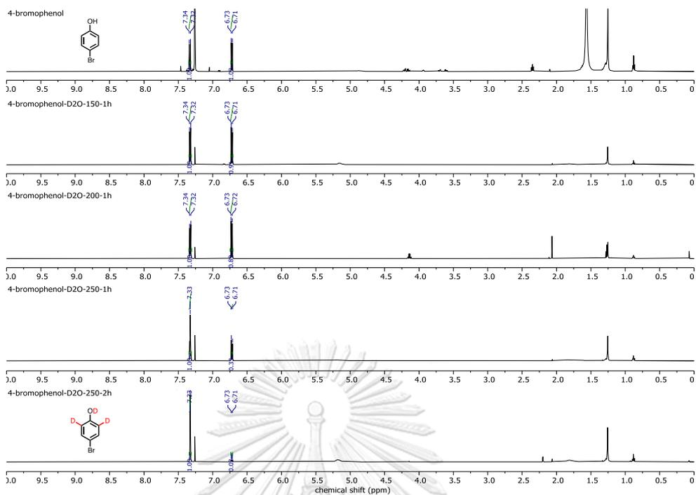
Figure A1  $^1\text{H}$  NMR (500 MHz,  $\text{CDCl}_3$ ) NMR spectrum of the HDx reaction of 4-bromophenol at 150-250  $^\circ\text{C}$  for 1-2 h
