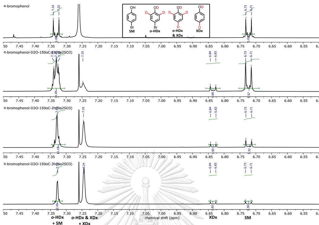
**Figure 3.25**  $^1\text{H}$  NMR spectra of XDx of 4-bromophenol mediated by  $\text{Na}_2\text{SO}_3$  in  $\text{D}_2\text{O}$  under hydrothermal conditions with different the reaction time
