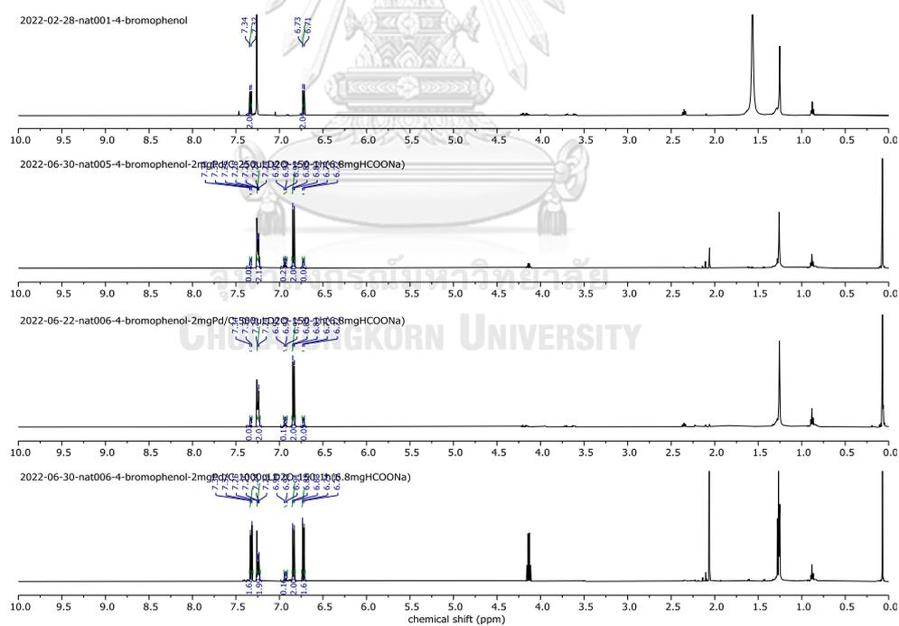
**Figure A52**  $^1\text{H}$  NMR (500 MHz,  $\text{CDCl}_3$ ) NMR spectrum of the XDi reaction of 4-bromophenol with various amount of  $\text{D}_2\text{O}$  at 150 °C for 1 h
