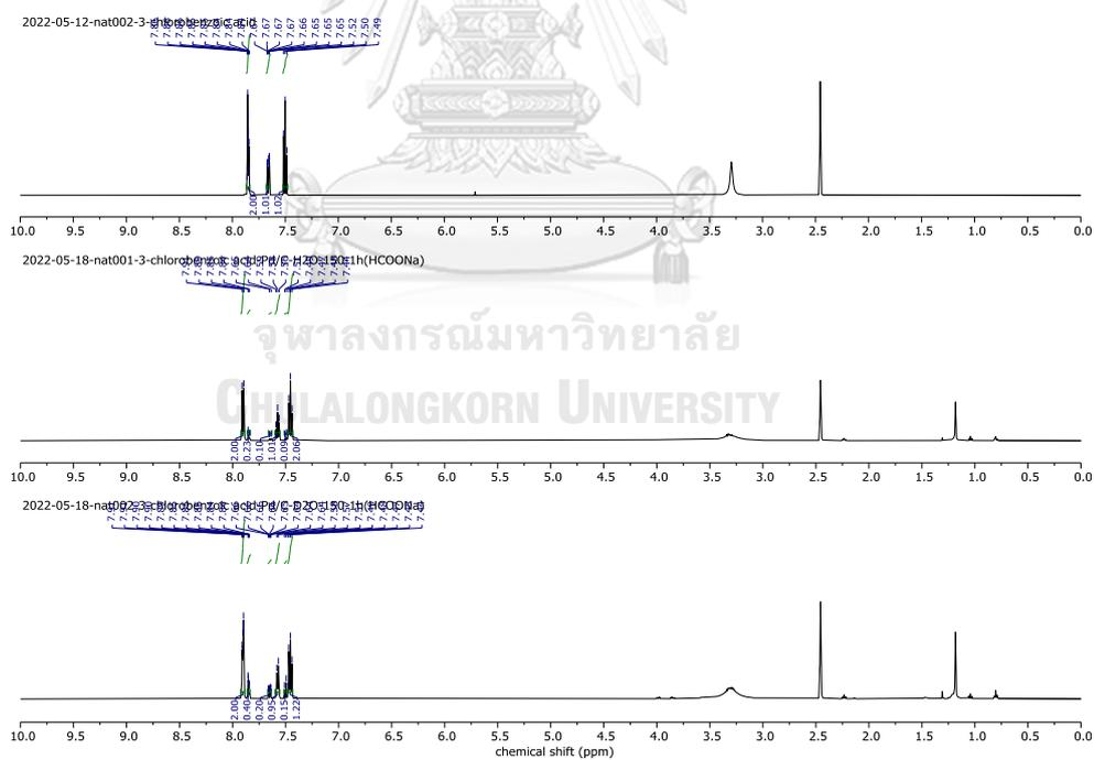
Figure A60  $^1\text{H}$  NMR (500 MHz,  $\text{DMSO}-d_6$ ) NMR spectrum of the XHx and XDx reaction of 3-chlorobenzoic acid with 0.15 mmol HCOONa and Pd/C at 150 °C for 1 h
