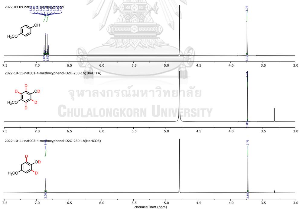
**Figure A8**  $^1\text{H}$  NMR (500 MHz,  $\text{D}_2\text{O}$ ) NMR spectrum of the HDx reaction of 4-methoxyphenol in the presence of TFA and  $\text{NaHCO}_3$  at 230 °C for 1 h
