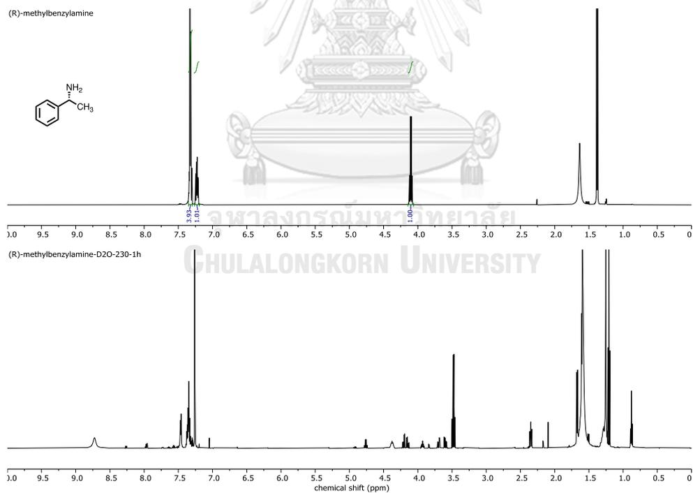
**Figure A26**  $^1\text{H}$  NMR (500 MHz,  $\text{CDCl}_3$ ) NMR spectrum of the HDx reaction of  $\alpha$ -methylbenzylamine at 230 °C for 1 h
