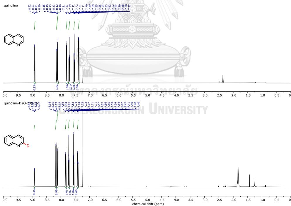
Figure A6  $^1\text{H}$  NMR (500 MHz,  $\text{CDCl}_3$ ) NMR spectrum of the HDx reaction of quinoline at 230 °C for 1 h
