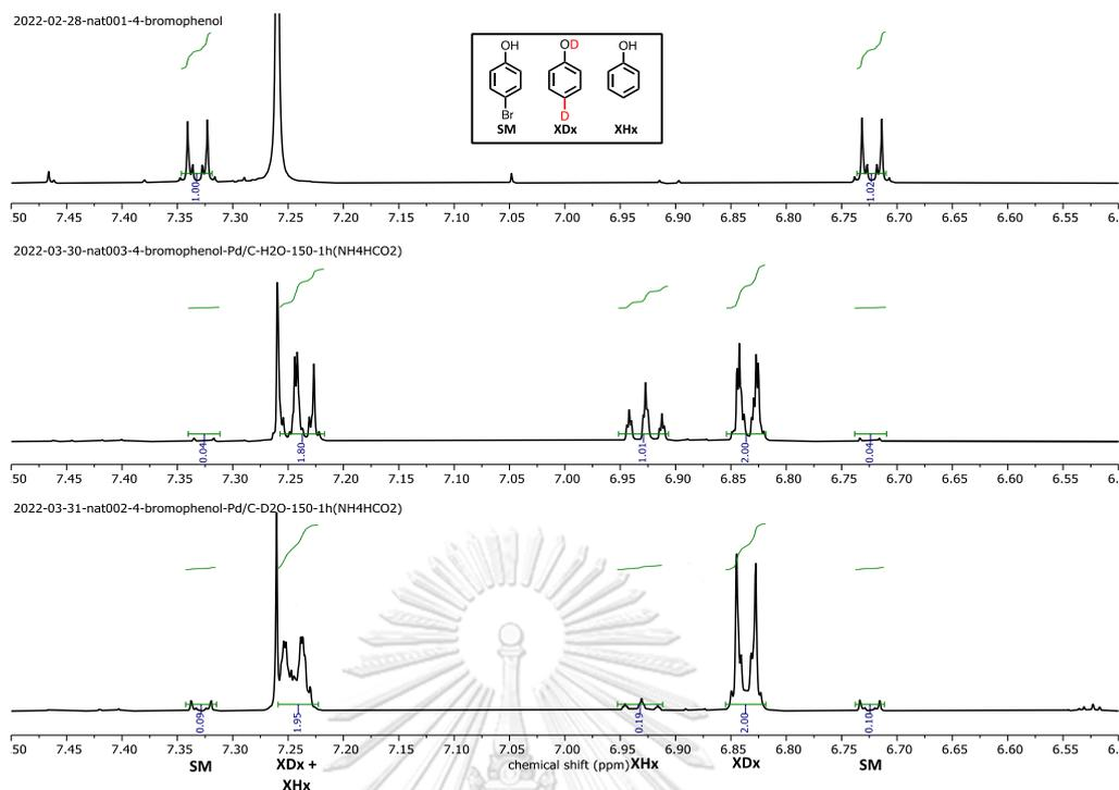
**Figure 3.28**  $^1\text{H}$  NMR spectra of the reaction products from the XDx and XHx of 4-bromophenol mediated by  $\text{HCOONH}_4$  and Pd/C in  $\text{H}_2\text{O}$  and  $\text{D}_2\text{O}$  under hydrothermal conditions
