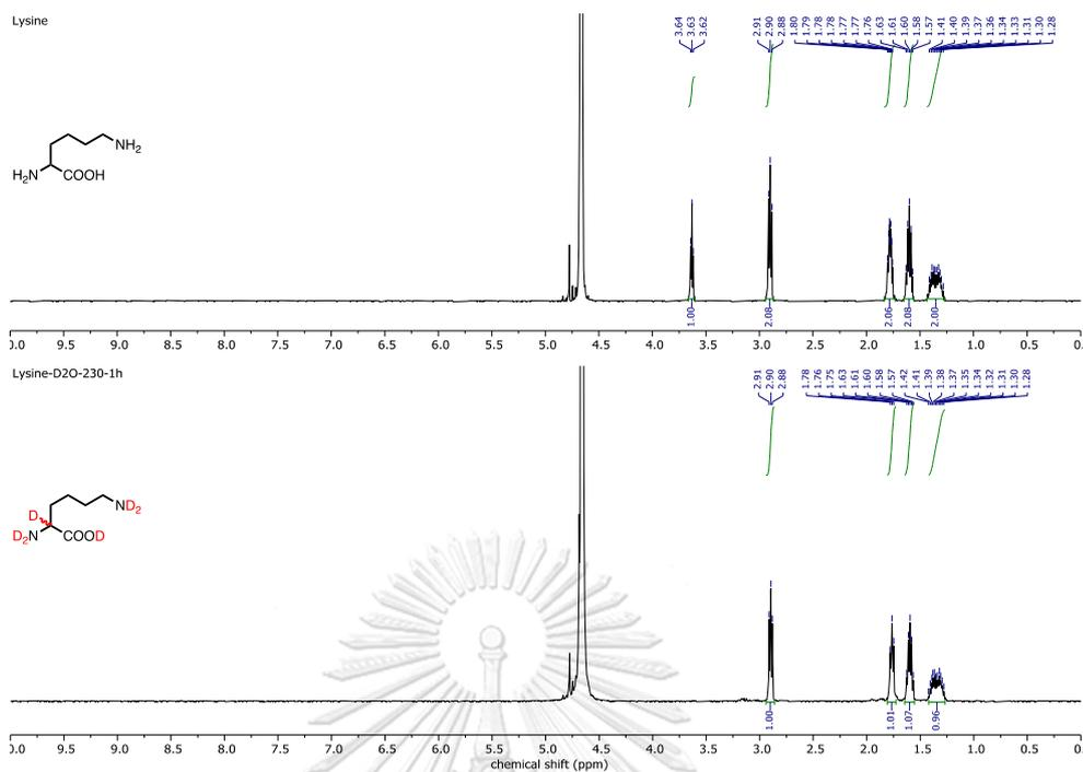
Figure A15  $^1\text{H}$  NMR (500 MHz,  $\text{D}_2\text{O}$ ) NMR spectrum of the HDx reaction of L-lysine at 230 °C for 1 h
