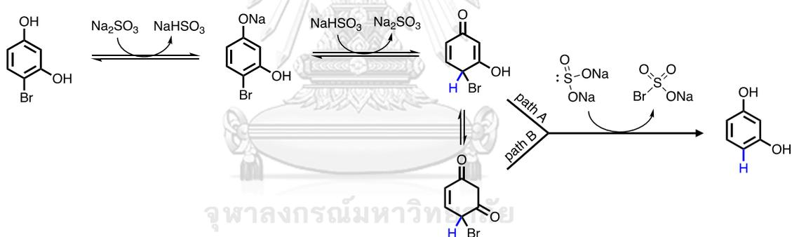
**Figure 1.21** Proposed mechanism of the debromination of 4-bromoresorcinol<sup>36</sup>
