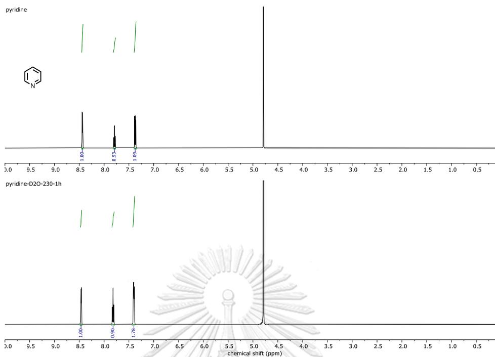
Figure A27  $^1\text{H}$  NMR (500 MHz,  $\text{D}_2\text{O}$ ) NMR spectrum of the HDx reaction of pyridine at 230 °C for 1 h
