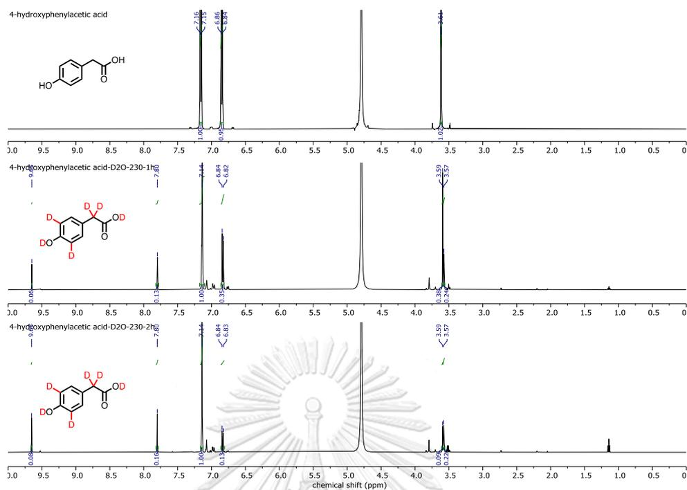
Figure A11  $^1\text{H}$  NMR (500 MHz,  $\text{D}_2\text{O}$ ) NMR spectrum of the HDx reaction of 4-hydroxyphenylacetic acid at 230 °C for 1-2 h
