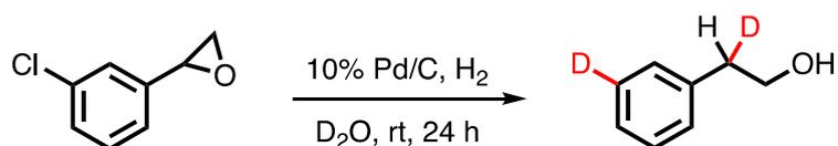
**Figure 1.11** HDx of 2-(3-chlorophenyl)oxirane with H<sub>2</sub> gas and D<sub>2</sub>O in the presence of 10% Pd/C<sup>26</sup>
