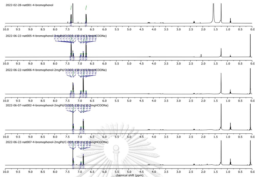
Figure A49  $^1\text{H}$  NMR (500 MHz,  $\text{CDCl}_3$ ) NMR spectrum of the XDx reaction of 4-bromophenol with various amount of HCOONa at 150 °C for 1 h
