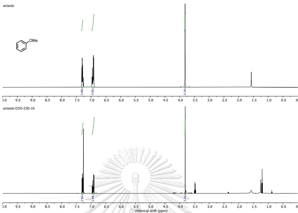
Figure A19  $^1\text{H}$  NMR (500 MHz,  $\text{CDCl}_3$ ) NMR spectrum of the HDx reaction of anisole at 230 °C for 1 h
