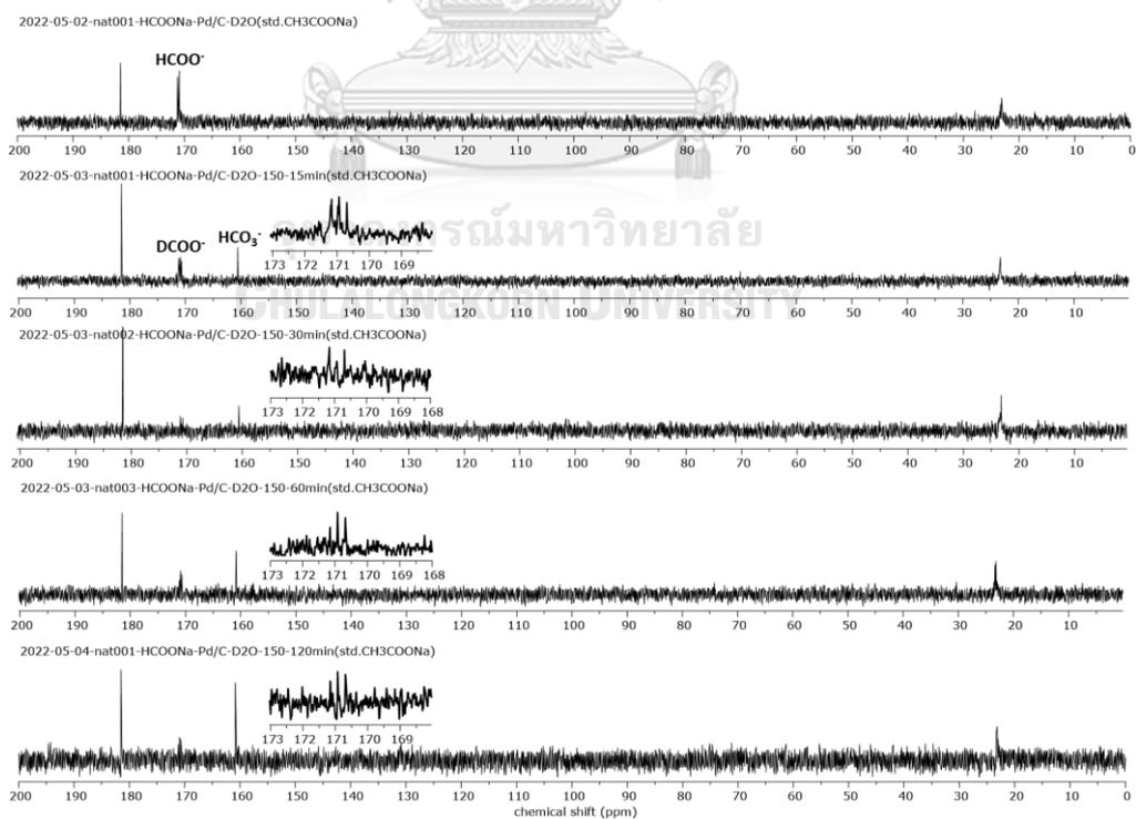
Figure 3.37  $^{13}\text{C}$  NMR spectra of the reaction products from the HDx of HCOONa in  $\text{D}_2\text{O}$  with  $\text{CH}_3\text{COONa}$  under hydrothermal conditions with different reaction time
