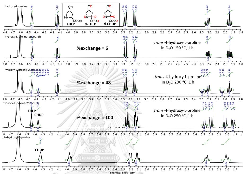
**Figure 3.3**  $^1\text{H}$  NMR spectra of the HDx reaction of *trans*-4-hydroxy-L-proline at different temperatures
