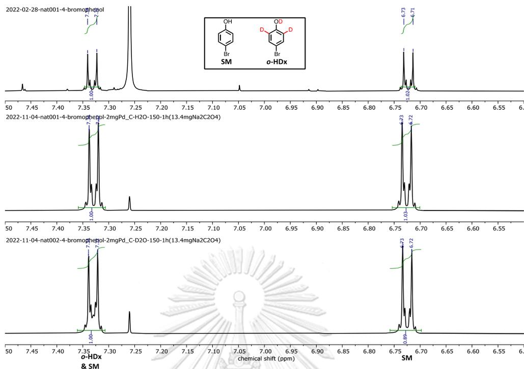
**Figure 3.39**  $^1\text{H}$  NMR spectra of the reaction products from the XHx and XDx of 4-bromophenol in the presence of  $\text{Na}_2\text{C}_2\text{O}_4$
