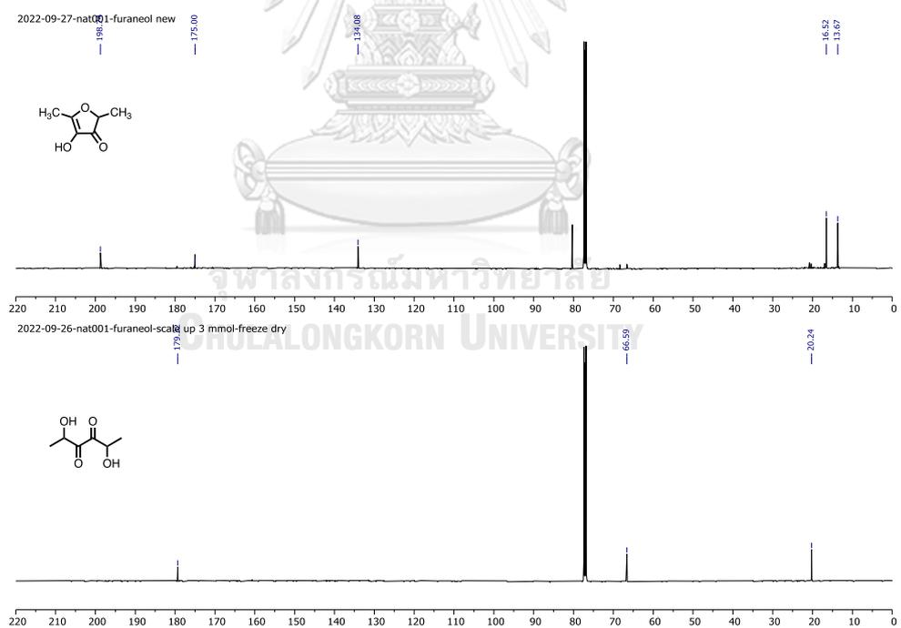
**Figure A40**  $^{13}\text{C}$  NMR (126 MHz,  $\text{CDCl}_3$ ) NMR spectrum of furaneol and 2,5-dihydroxyhexane-3,4-dione
