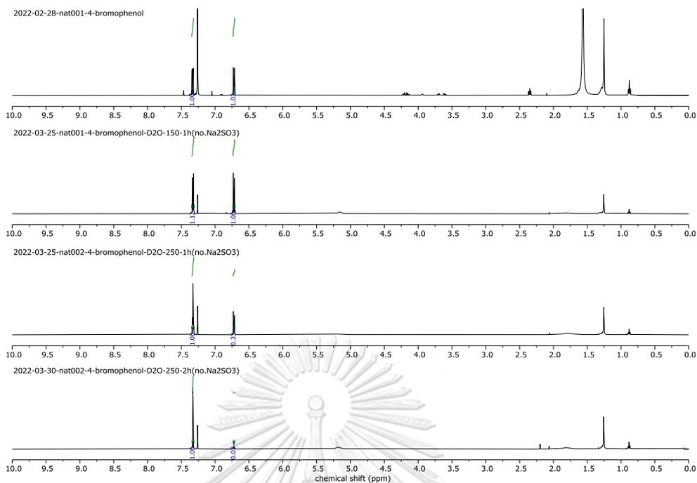
**Figure A47**  $^1\text{H}$  NMR (500 MHz,  $\text{CDCl}_3$ ) NMR spectrum of the XDx reaction of 4-bromophenol in the absence of  $\text{Na}_2\text{SO}_3$  at 150-250 °C for 1-2 h
