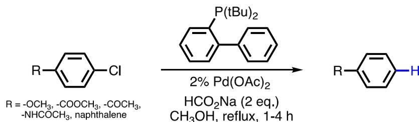
**Figure 1.18** Hydrodechlorination of aryl chloride in with sodium formate in the presence of a homogeneous palladium catalyst
