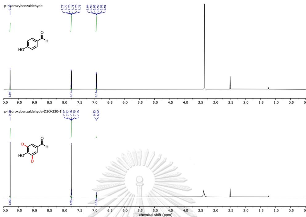
Figure A5  $^1\text{H}$  NMR (500 MHz,  $\text{DMSO}-d_6$ ) NMR spectrum of the HDx reaction of *p*-hydroxybenzaldehyde at 230 °C for 1 h
