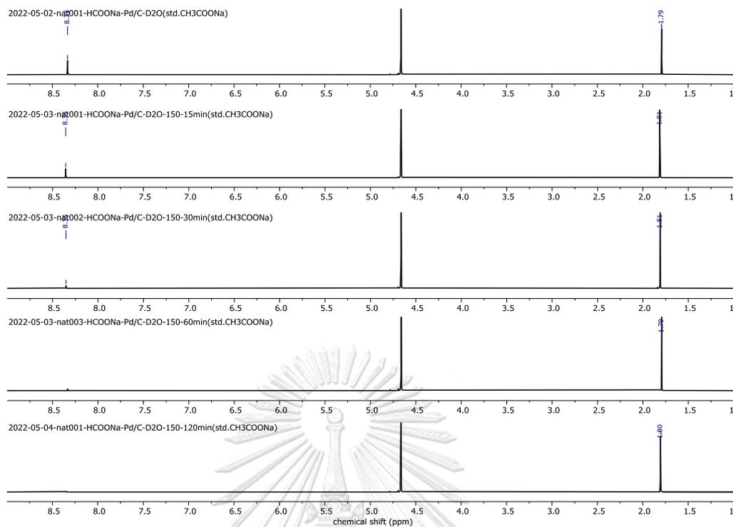
Figure 3.36  $^1\text{H}$  NMR spectra of the reaction products from the HDx of HCOONa in  $\text{D}_2\text{O}$  with  $\text{CH}_3\text{COONa}$  under hydrothermal conditions with different reaction time
