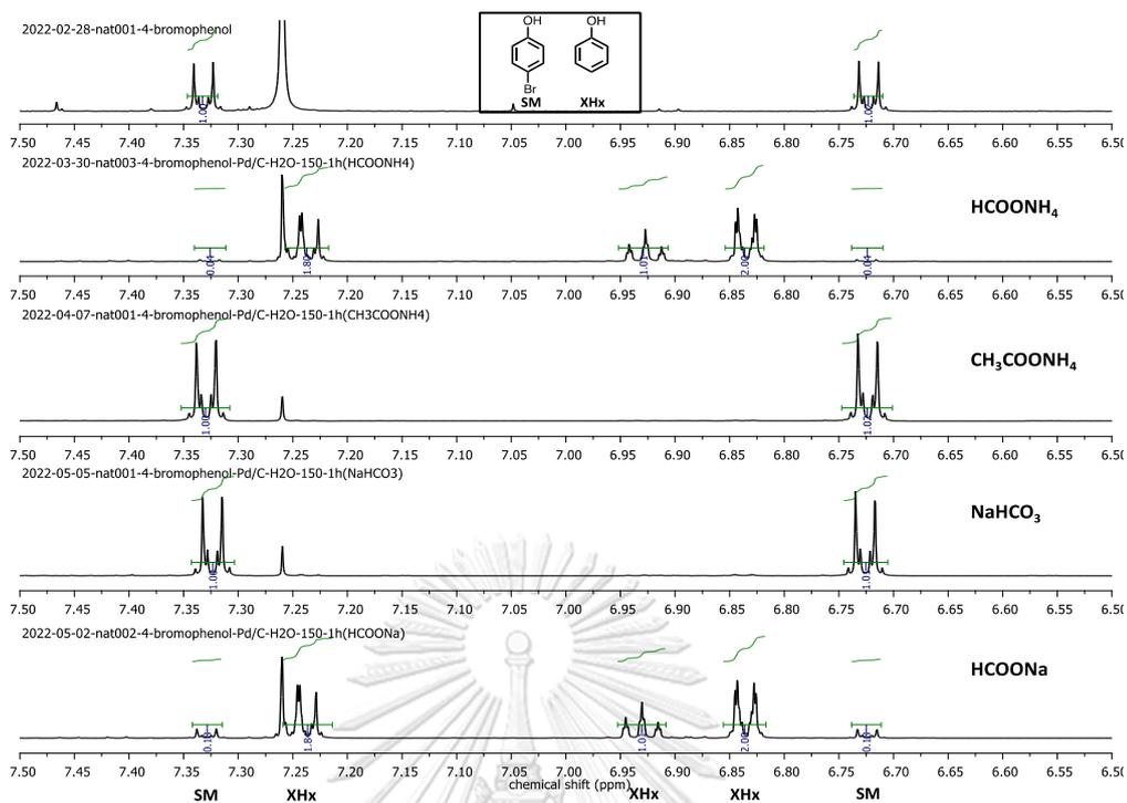
Figure 3.30  $^1\text{H}$  NMR spectra of the reaction products from the XHx of 4-bromophenol with different additives in  $\text{H}_2\text{O}$
