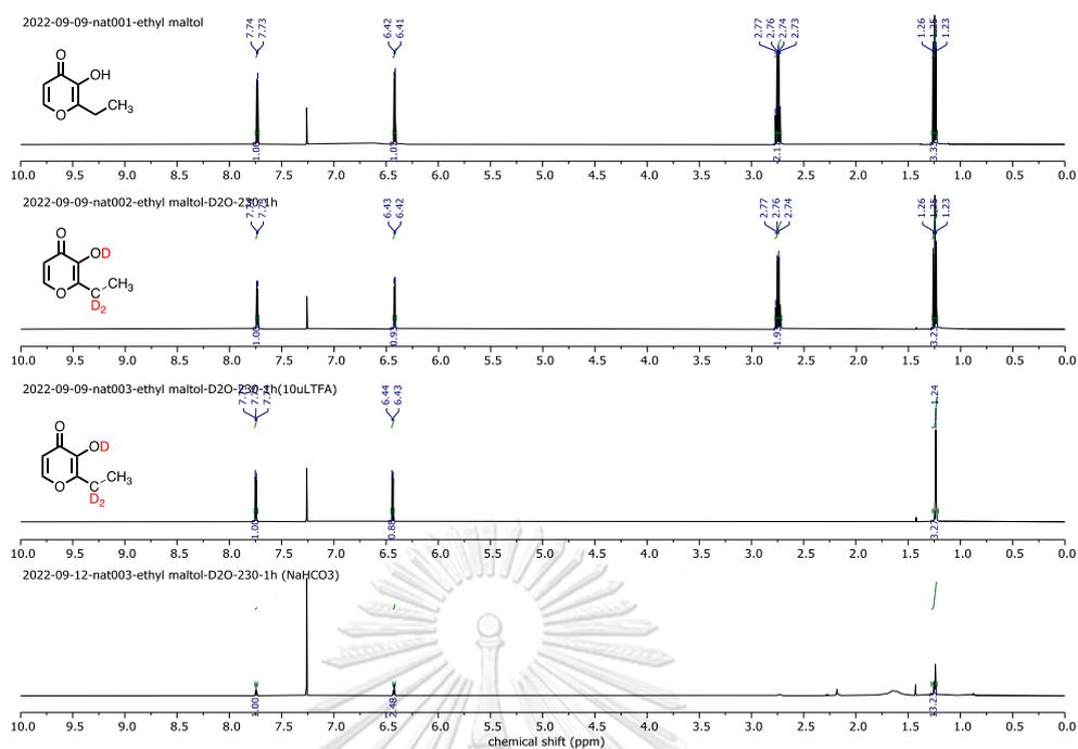
Figure A35  $^1\text{H}$  NMR (500 MHz,  $\text{CDCl}_3$ ) NMR spectrum of the HDx reaction of ethyl maltol at 230 °C for 1 h under neutral, acid, and base conditions
