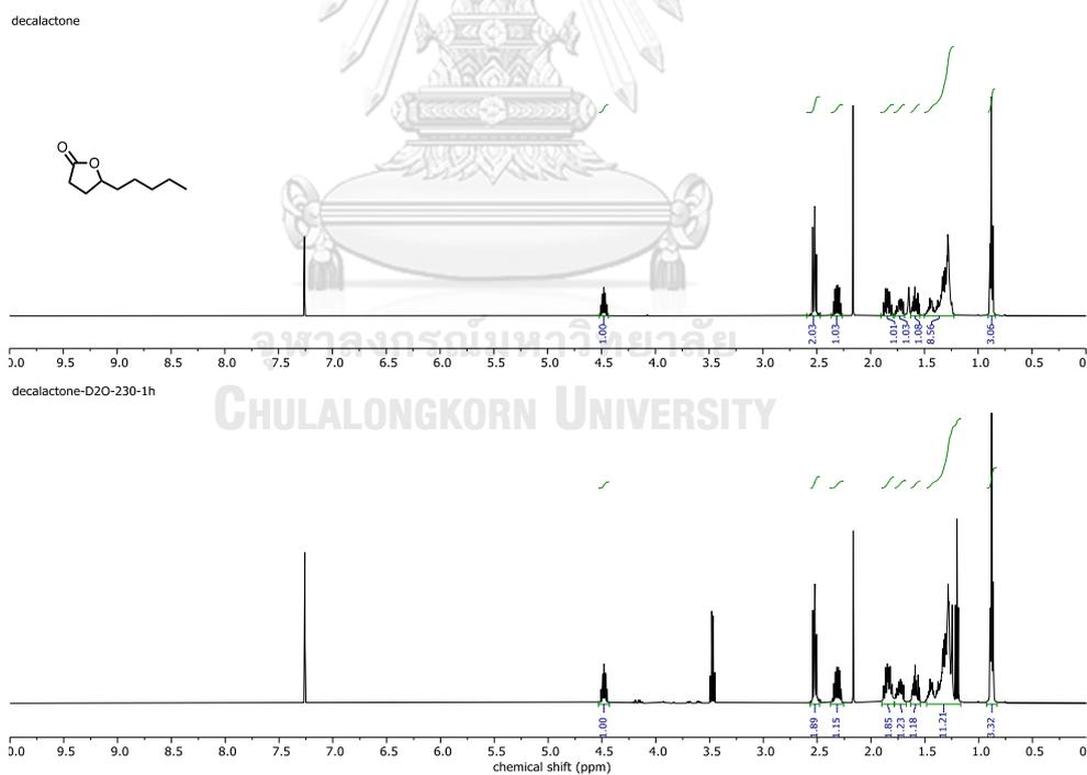
Figure A18  $^1\text{H}$  NMR (500 MHz,  $\text{CDCl}_3$ ) NMR spectrum of the HDx reaction of decalactone at 230 °C for 1 h
