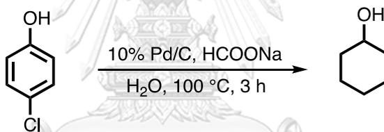
**Figure 1.17** Dearomatization of 4-chlorophenol in water with HCOONa and catalytic 10% Pd/C at 100 °C for 3 h
