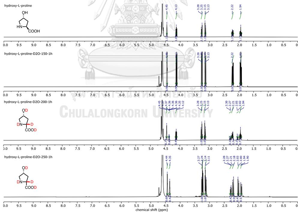
Figure A12  $^1\text{H}$  NMR (500 MHz,  $\text{D}_2\text{O}$ ) NMR spectrum of the HDx reaction of *trans*-4-hydroxy-L-proline at 150-250 °C for 1 h
