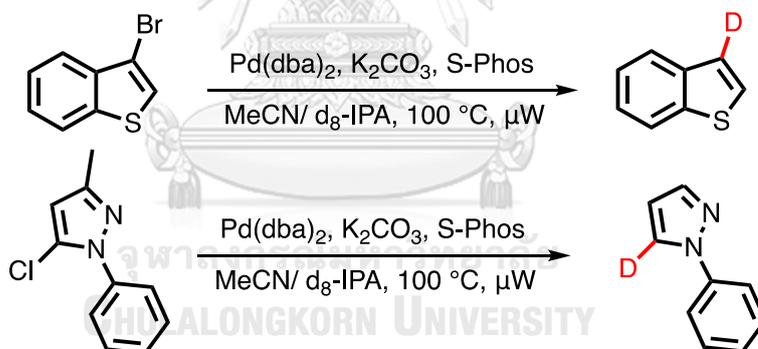
**Figure 1.23** Deuteration of 3-bromo-1-benzothiophene and 5-chloro-3-methyl-1-phenylpyrazole with  $\text{Pd}(\text{dba})_2$  in  $d_8$ -IPA under microwave condition
