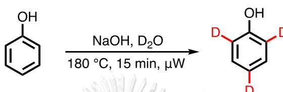
**Figure 1.6** HDx of phenol using NaOH in D<sub>2</sub>O under microwave irradiation
