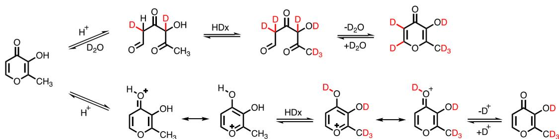
Figure 3.15 A proposed mechanism of the HDx of maltol
