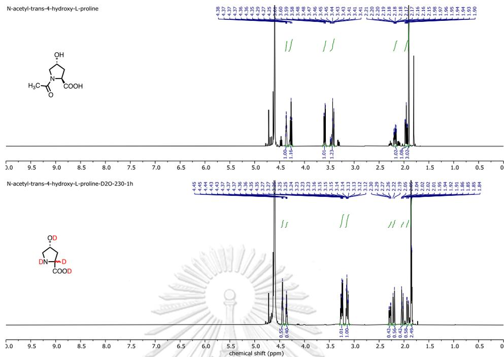
Figure A13 <sup>1</sup>H NMR (500 MHz, D<sub>2</sub>O) NMR spectrum of the HDx reaction of *N*-acetyl-*trans*-4-hydroxy-L-proline at 230 °C for 1 h
