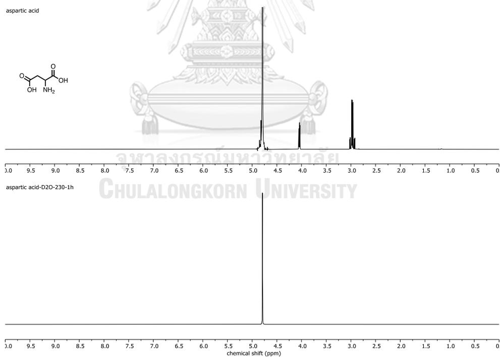
**Figure A22**  $^1\text{H}$  NMR (500 MHz,  $\text{D}_2\text{O}$ ) NMR spectrum of the HDx reaction of L-aspartic acid at 230 °C for 1 h
