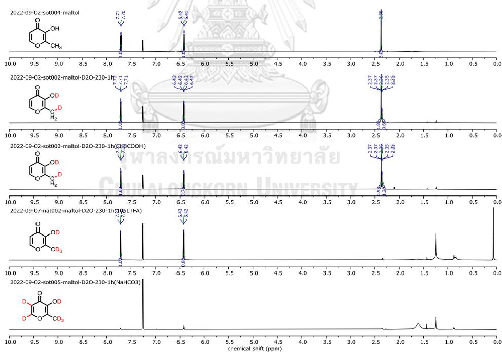
Figure A30  $^1\text{H}$  NMR (500 MHz,  $\text{CDCl}_3$ ) NMR spectrum of the HDx reaction of maltol at 230 °C for 1 h under neutral, acid, and base conditions
