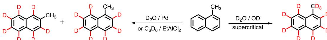
**Figure 1.12** Deuteration of 1-methylnaphthalene in the absence and presence of D<sub>2</sub>O/Pd or ethylaluminium dichloride/benzene-*d*<sub>6</sub> under supercritical condition
