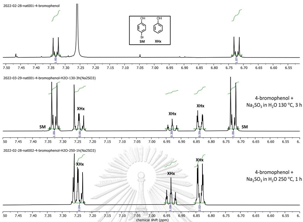
**Figure 3.23**  $^1\text{H}$  NMR spectra of debromination of 4-bromophenol in water under hydrothermal condition at 130 °C for 3 h and 250 °C for 1 h
