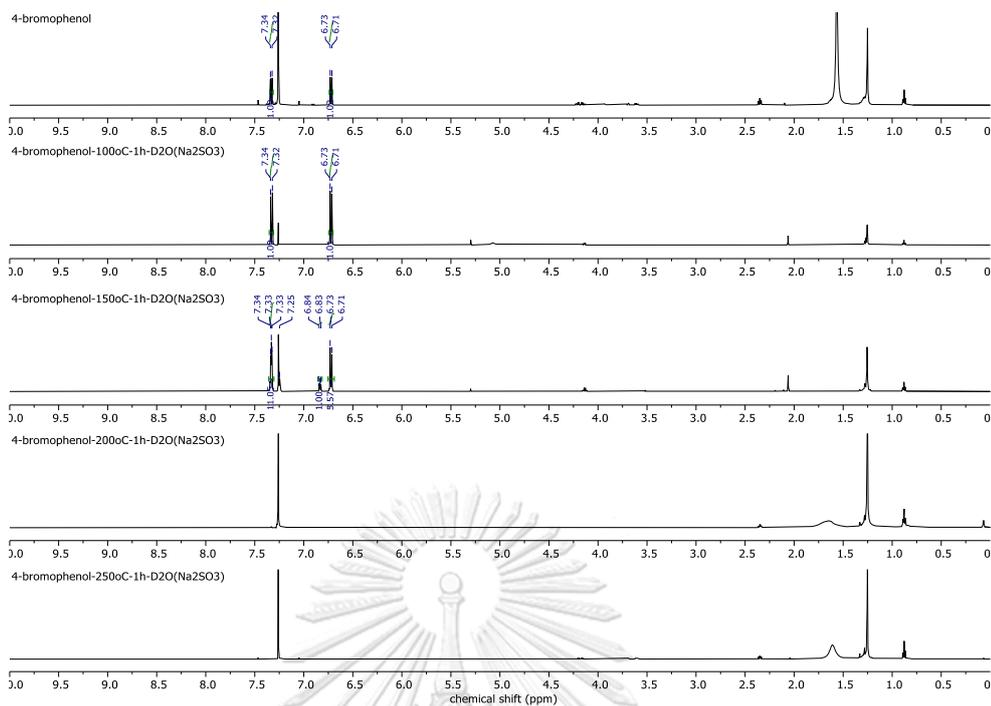
Figure A45  $^1\text{H}$  NMR (500 MHz,  $\text{CDCl}_3$ ) NMR spectrum of the XDx reaction of 4-bromophenol in the presence of  $\text{Na}_2\text{SO}_3$  with various amount of reaction temperature for 1 h
