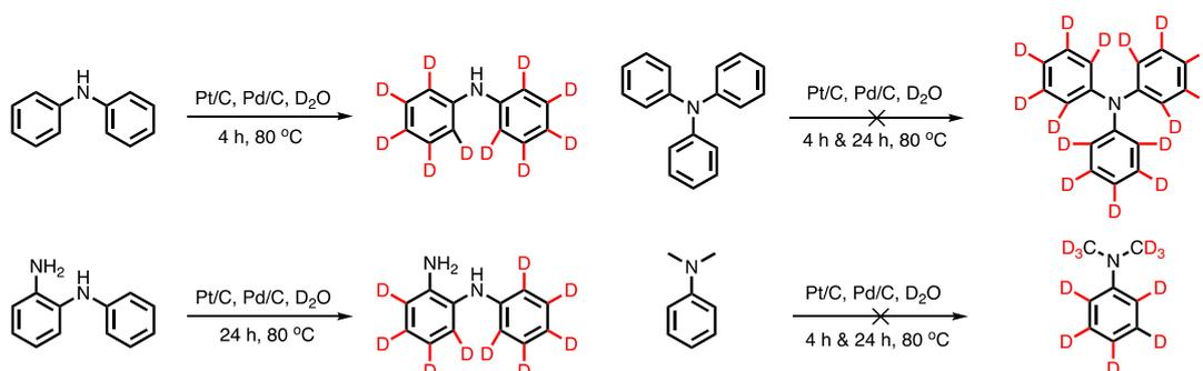
**Figure 1.7** HDx of arylamine in  $D_2O$  catalyzed by Pd/C or Pt/C
