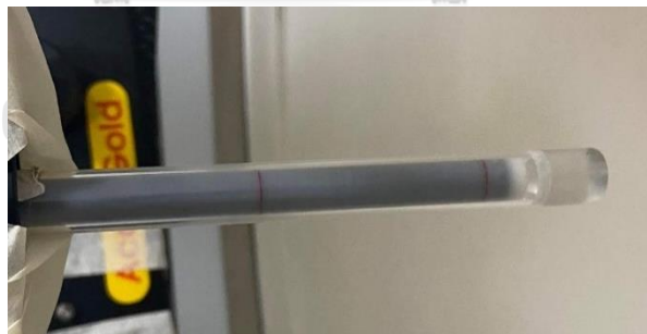
Figure 3.7 The ionization chamber for measurement of Computed Tomography Dose Index (CTDI)
