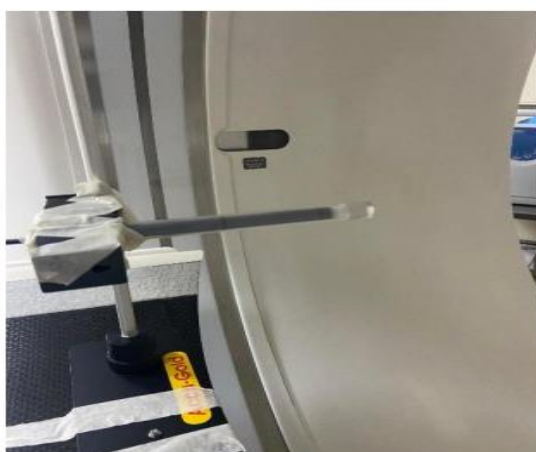
Figure B-12 CTDI_{100} in air measurement using 100 mm pencil ion chamber.
