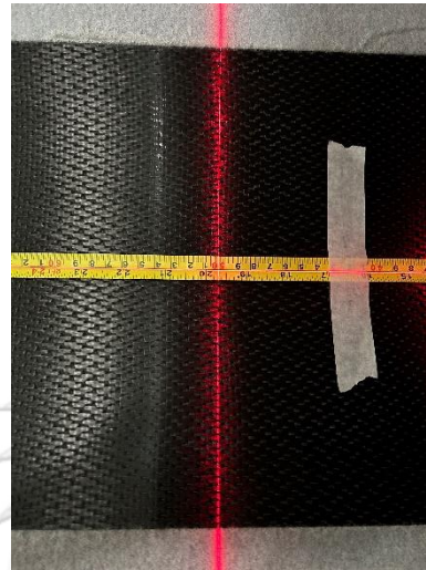
Figure B-1. The measurement of scan localization light accuracy.
