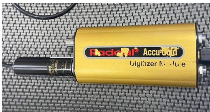
Figure 3.8 Radcal® Accu-Gold+ digitizer module.
