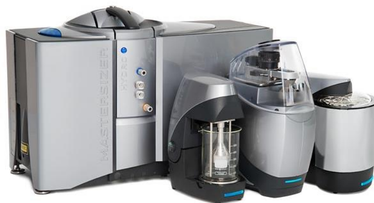
Figure 14 Laser particle size distribution analyzer - MALVERN Mastersizer 3000 (STREC Chula) that used for grain size analysis.
