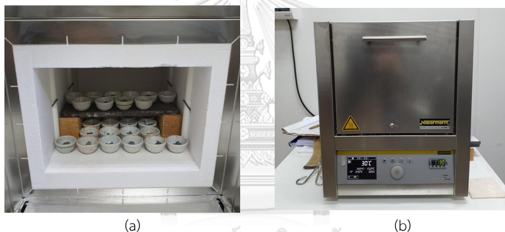
Figure 13 LOI testing (a) sediment sample in ceramic pot and (b) high temperature muffle furnace.
