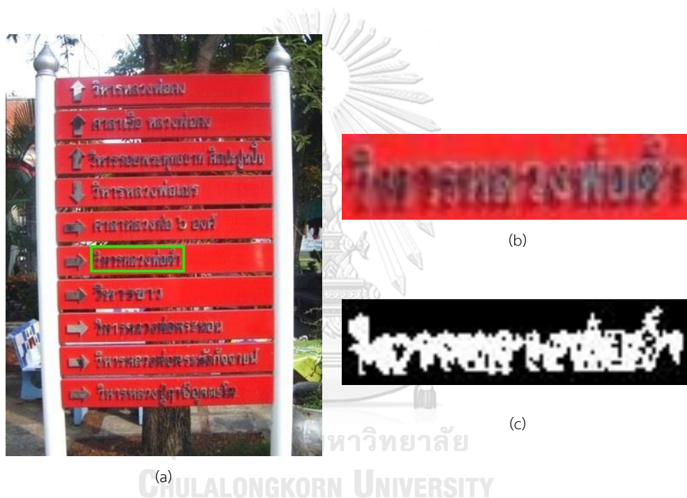
Figure 29 (a) Sample of detected text instance. (b) Cropped detected text instance. (c) Simple thresholded result. As show in the figure, simple thresholding cannot distinguish cropped word into single individual character.
