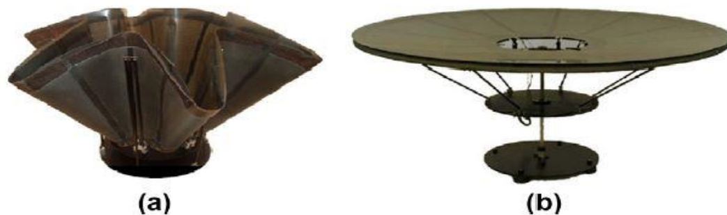
Figure 2.5 Shape-memory polymer composite-reflector: (a) pre-deformed shape and (b) recovered shape [24].
