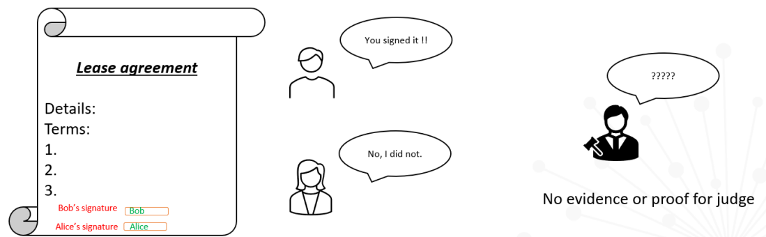
Figure 4 Not non-repudiation; the signer can deny any involvement with the contract. A good signature should be undeniable once signed.
