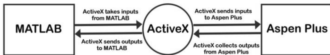
Figure 11 A block diagram illustrating the integration of Aspen Plus with MATLAB [29].
