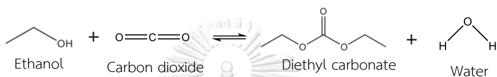
Figure 23 Reaction for producing DEC from EtOH and CO 2 .
