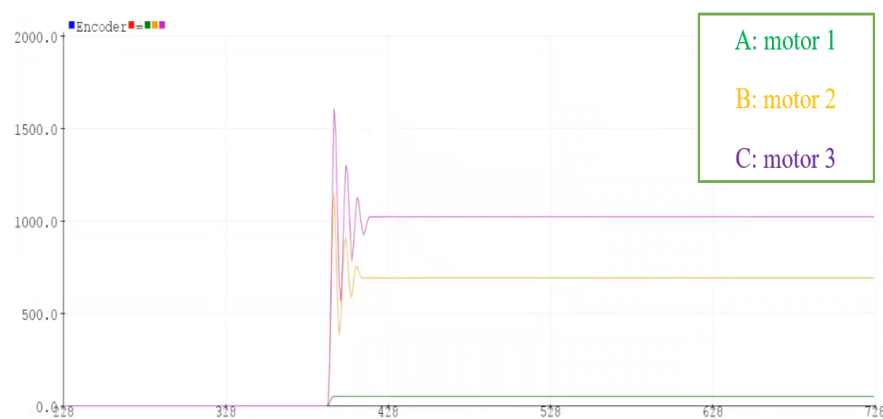
Fig. 7. Graph of the motor reaction after position control input
