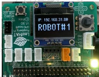
Fig. 29. OLED screen and LED output for single robot experiment
