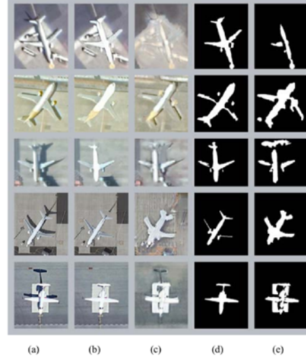
Figure 3. The five lowest score results: (a) Original image, (b) Manually shadow removal image (ground truth), (c) GAN generated of (a), (d) Aircraft shape of (b), (e) Aircraft shape of (c)
