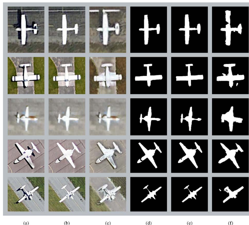
Figure 4.2.1 The five highest score results: (a) Original image, (b) Manually shadow removal image (ground truth), (c) GAN generated of (a), (d) Aircraft shape of (b), (e) Aircraft shape of (c), (f) Aircraft shape from Meeboonmak [4]
