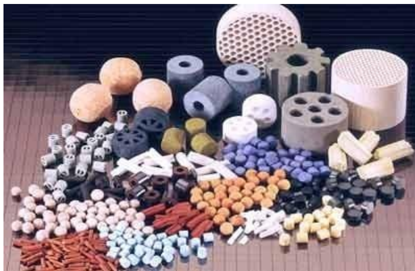
Figure 2.3 Various catalyst shapes using the industrial [29]
