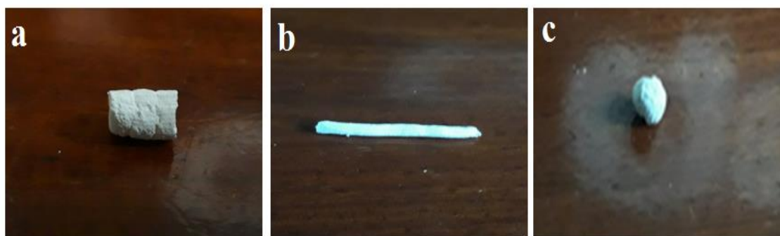
Figure 4.6 Extruded CaO catalyst pellets with different shapes (a) short cylindrical (SCY), (b) long cylindrical shapes (LCY) and (c) spherical shape (SHL)
