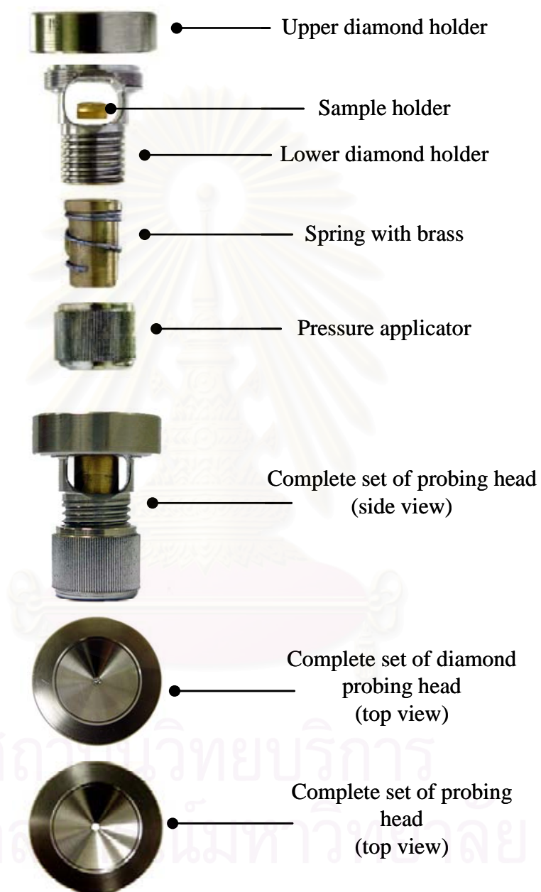
Figure 1 Composition of homemade accessory for diamond probing head.
