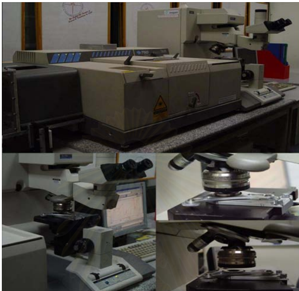
Figure 3.2 The homemade diamond \mu ATR accessory mounted onto the infrared microscope.
