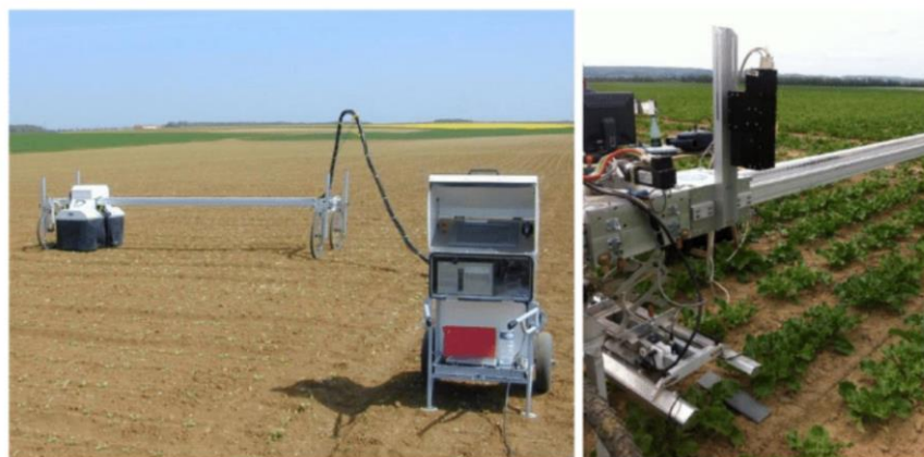
Figure 9 Phenotyping platform with the hyperspectral camera for N content detection (Wang et al. , 2020).
