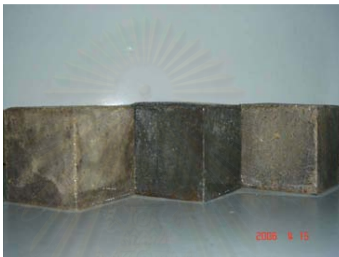
Figure C-1 Cement Mortars Containing Recycled Aggregate
