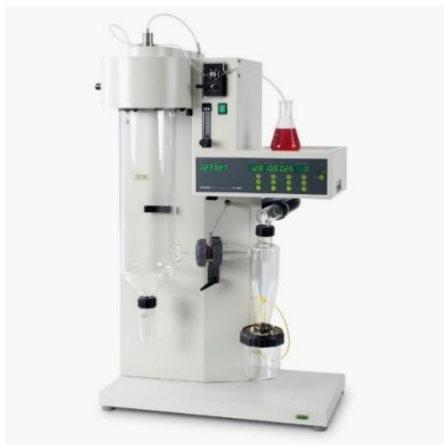
Figure 9 Mini spray dryer B-290, BUCHI (Thailand) Ltd.
