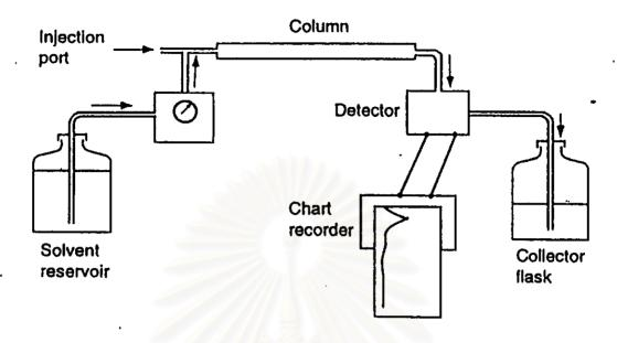
Figure 4.3 Basic Instrumentation for Gel Permeation Chromatography (GPC)
