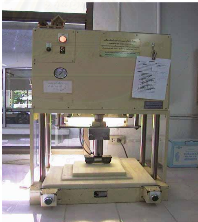
Figure 4.6 Photographic illustration of cutter for Tensile Testing.
