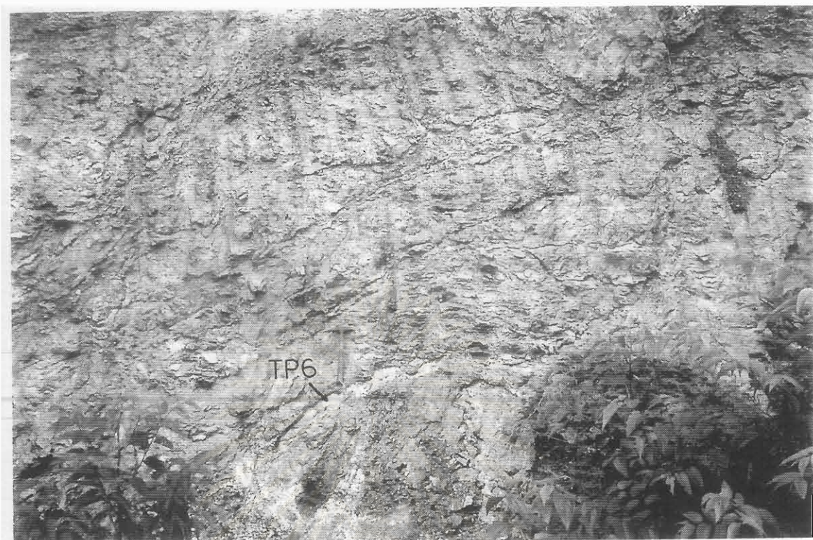
Figure 4.53 Road-cut, steep-cliff exposure of sheared and deformed siltstone interbedded with sandstone. Fault-gouge material (TP6) was collected from as semi-consolidated pale greenish yellow silt to clayey silt material.
