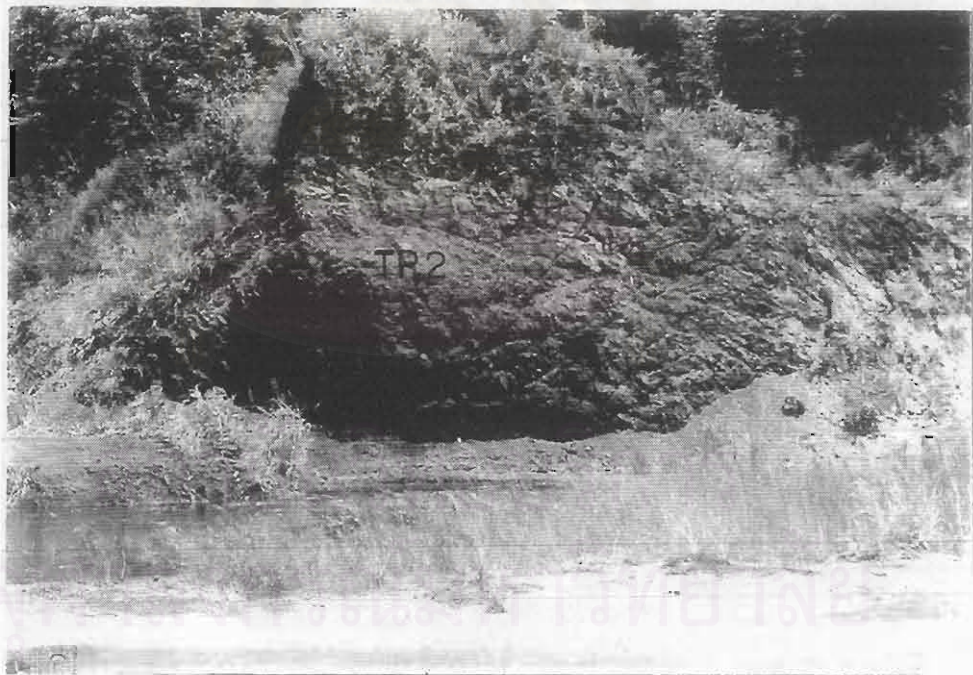
Figure 4.49 Road-cut exposure of weathered sheared and strongly deformed calcareous black shale on a road side from Thong Pha Phum to Sangkhla Buri, Ban Tha Madua, north Kanchanaburi. Sample no. TP2 is collected right at the arrowed mark.
