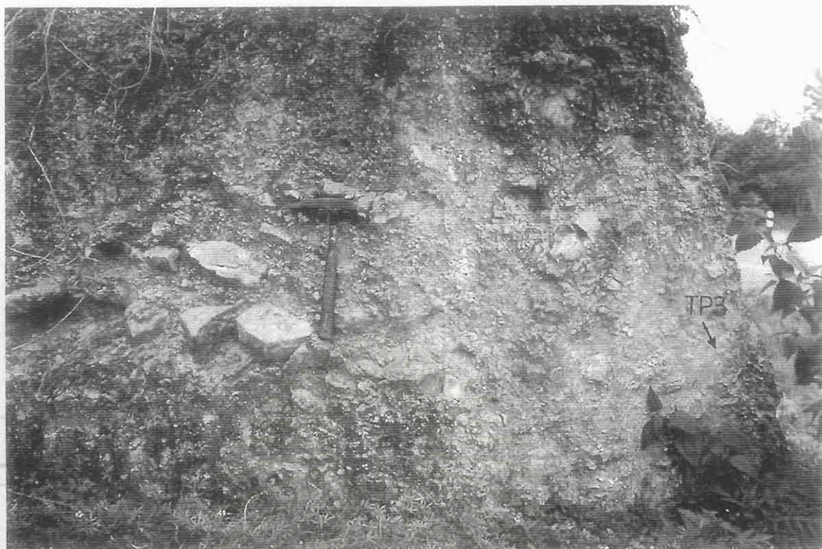
Figure 4.50 Road-cut exposure at the foot of Khao Wong limestone showing poorly sorted angular fragments of travertine with clay and silt matrix. Note that sample TP3 is collected for ESR dating.
