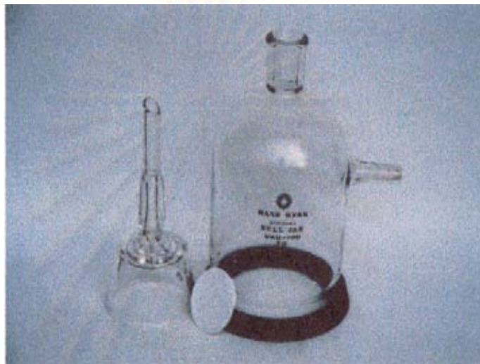
Figure 4.3 The vacuum filter
