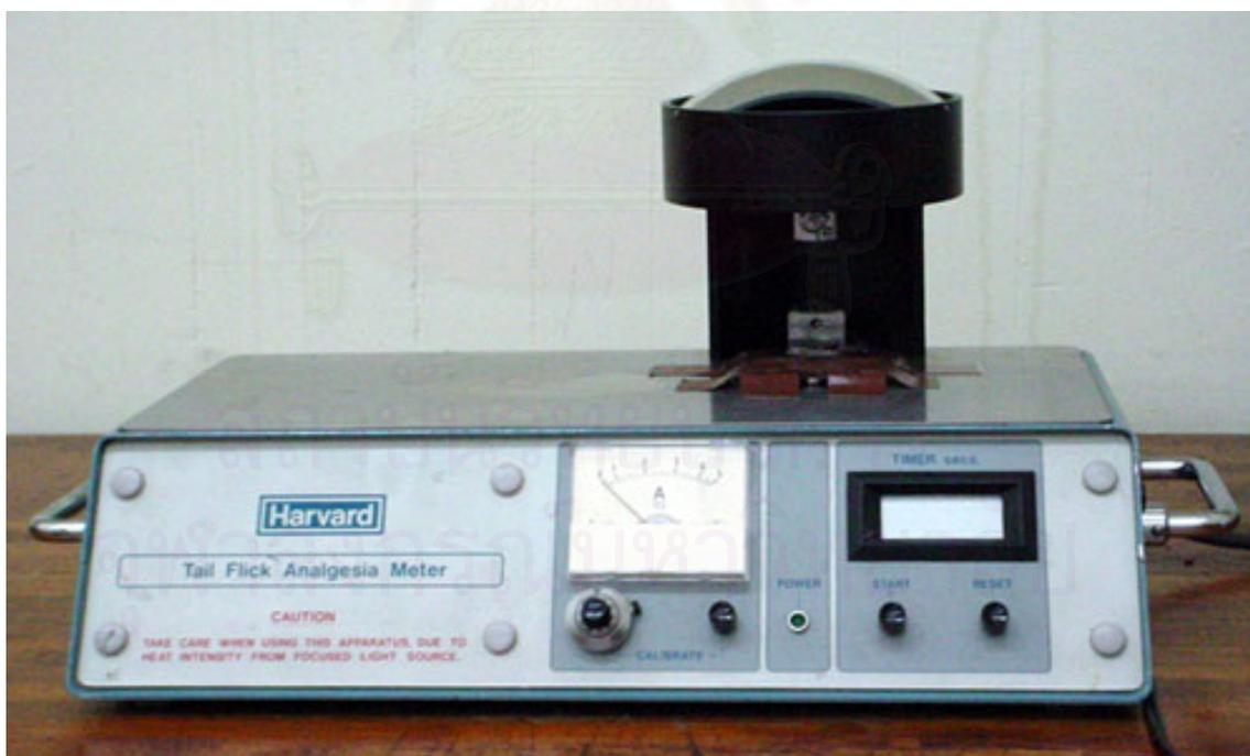
Figure 8 Photograph of a Harvard Tail Flick Analgesia Meter.
