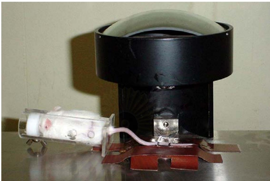
Figure 7 Photograph of a mouse on the device showing the focus of light beam.
