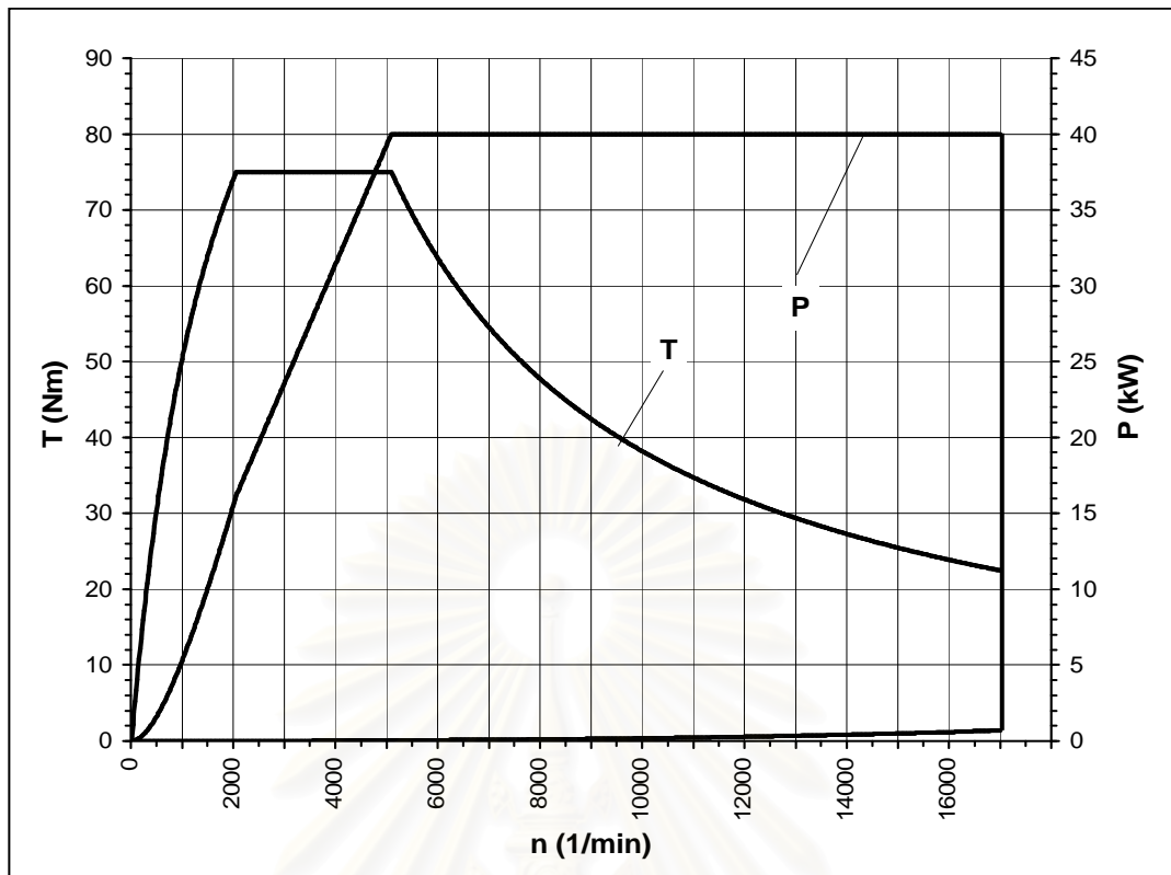
Figure C-2 Output and torque limit of AVL Alpha 40 dynamometer
