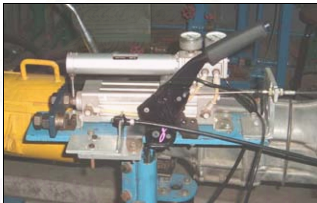
Figure 4–1 Pneumatic actuator SMC-SPCP-004 and mechanical throttling controller
