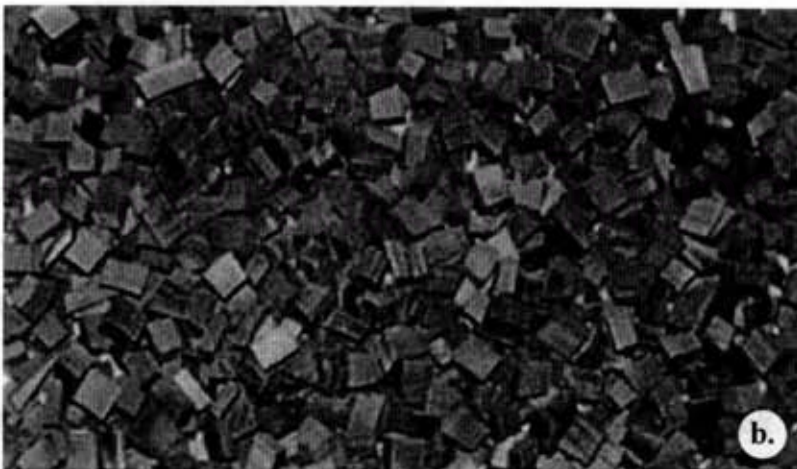
Figure 3.1 (a) used tires and (b) used tires size of 5 x 5 x 5 mm.
