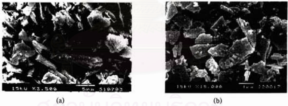
Fig. 4.12 SEM images of agglomerates (a) and dispersed DCPD crystals (b).
