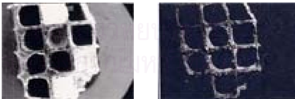
Figure 5.4 SEM photographs of supported beta zeolite
