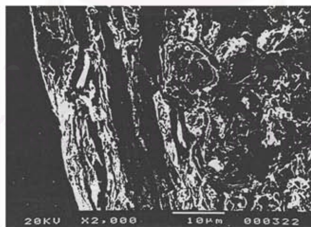
Figure 35 Photomicrographs of coated pellets Formulation 22 (10 % EC 100).
