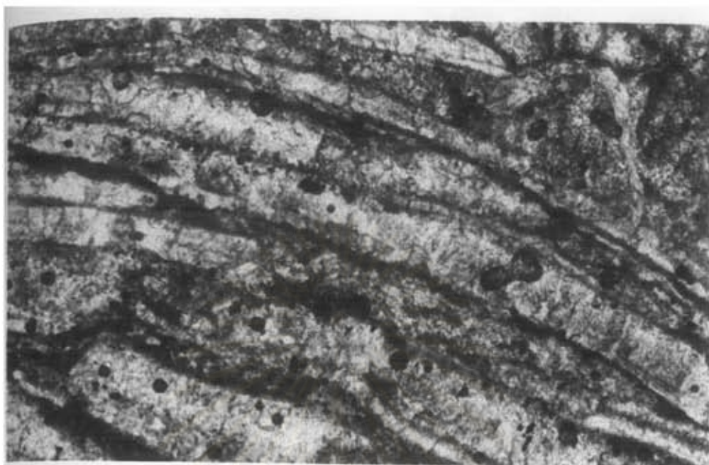
Figure 3.55 Photomicrograph of biomicrite (the Khlong Min formation, PT-1), showing preferred orientation of bioclasts with micrite envelopes infilled with neomorphic spar, crossed nicols, \times 40 .
