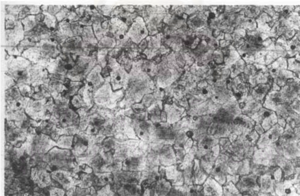
Figure 3.52 Photomicrograph of dolomite (the Sai Bon formation, KN1-7), showing mosaic of anhedral dolomite which replaced in the original limestone, crossed nicols, \times 40 .
